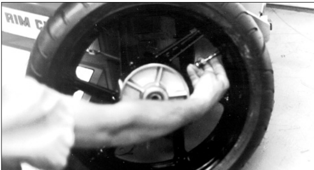
Figure 1 - Remove Valve Core to Deflate Tire
