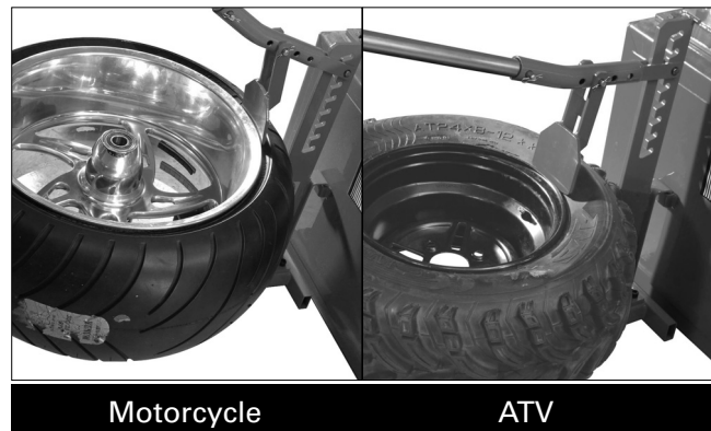
Figure 2 - Position Tire on Bead Loosener Shoe
