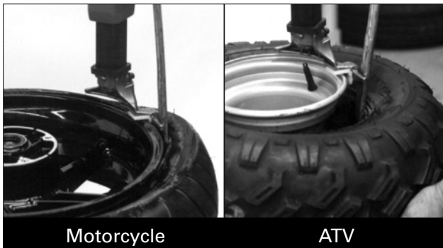
Figure 10 - Insert Bead Lifting Tool
