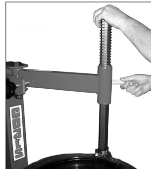
Figure 7 - Position Mount/Demount Tool
