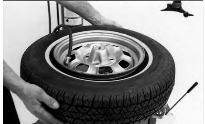
Figure 25 - Lift Tire Upwards for Bead Sealing
