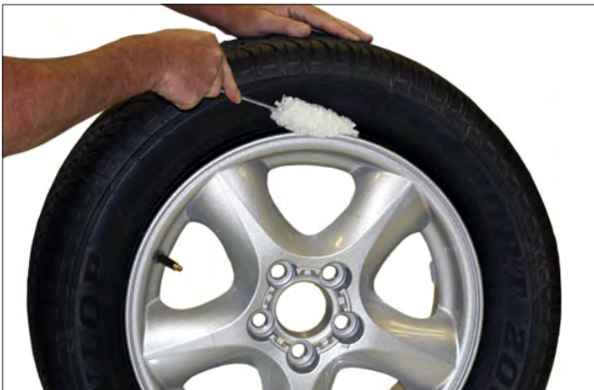
Figure 5 - Apply Rubber Lubricant to Tire Beads
