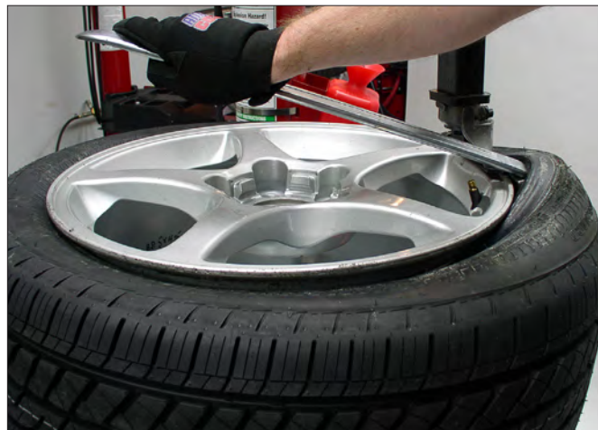
Figure 11 - Lift Bead Over Demount Tool
