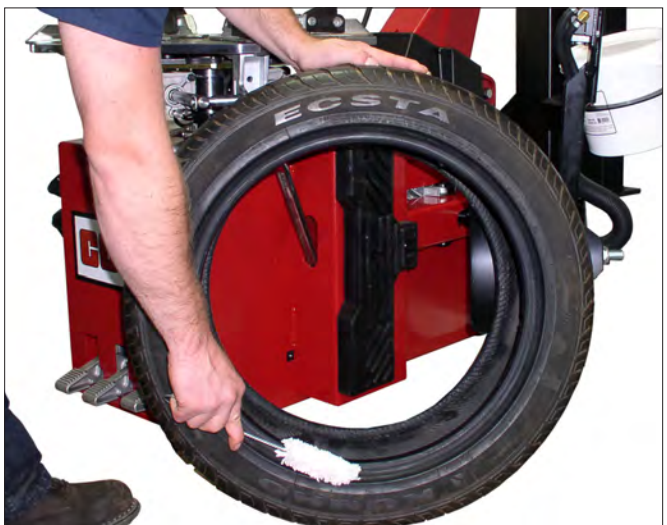
Figure 20 - Lubricate Tire Beads Liberally
