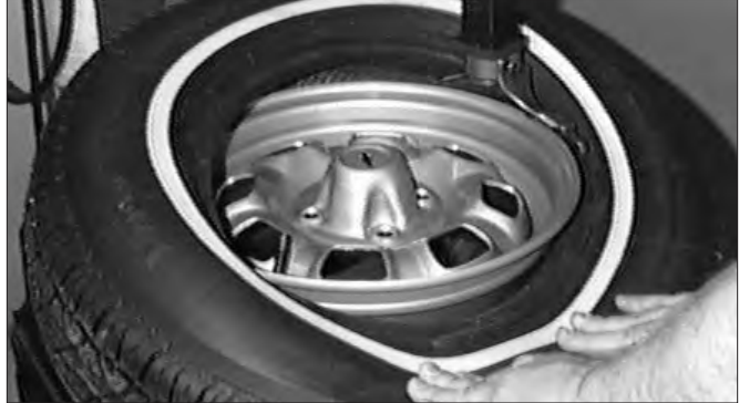
Figure 22- Mounting Top Bead
