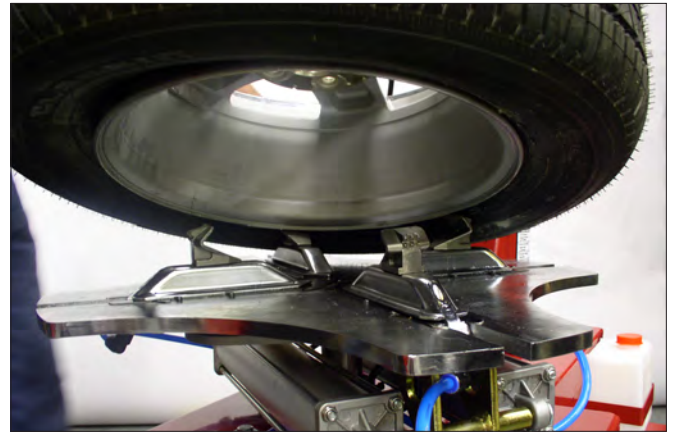
Figure 6 - Place Tire/Wheel Assembly on Table Top
