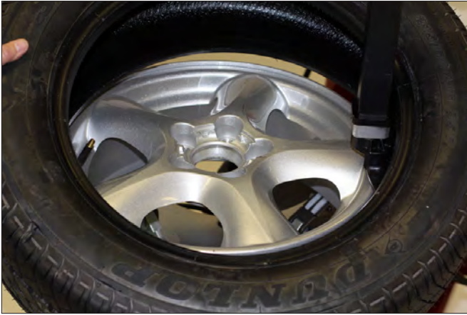
Figure 21 - Position Tire Against Duckhead® Mount Tool
