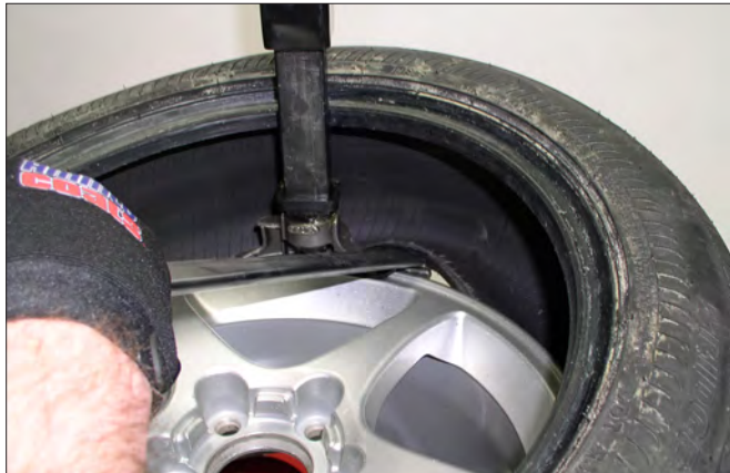
Figure 13- Guide Bead Over Tool Head
