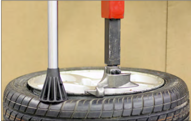
Figure 14 - Robo-Arm LR Foot Depressing Sidewall of Tire
