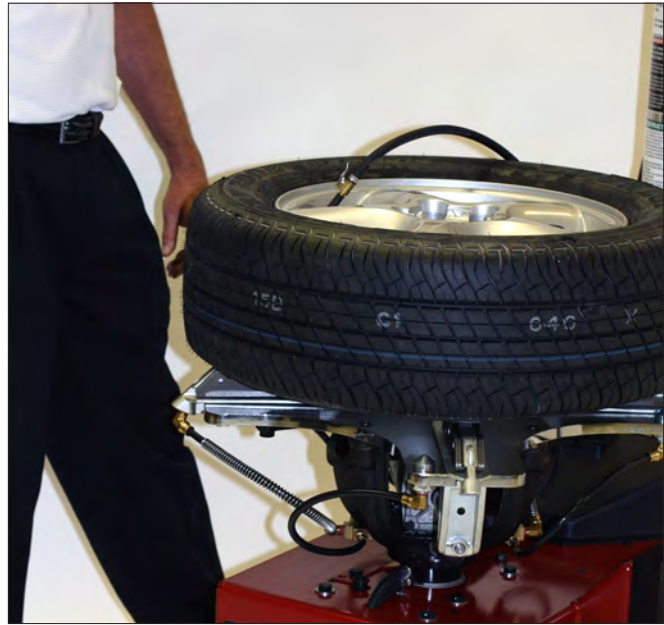
Figure 26 - Stand Back during Bead Seat
