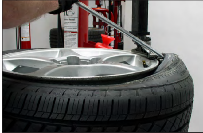
Figure 16 - Lift Bead Over Demount Tool
