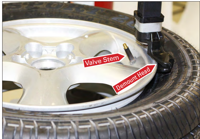
Figure 17 - Position Valve Stem Behind Demount Tool Tail
