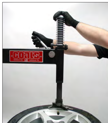
Figure 7 - Position Mount/Demount Tool
