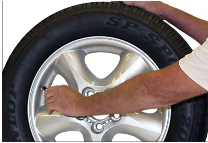
Figure 1 - Remove Valve Core to Deflate Tire
