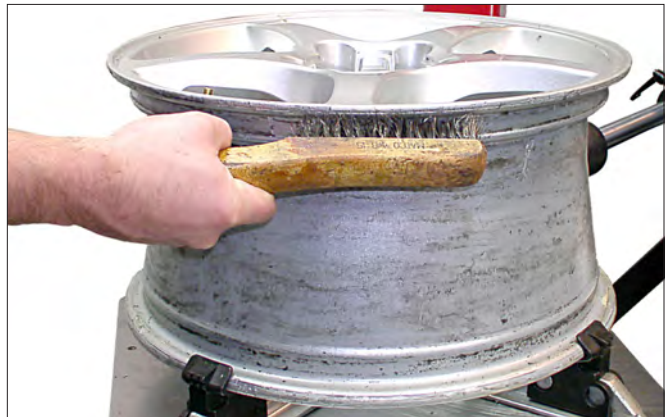
Figure 19 - Inspect and Clean the Wheel
