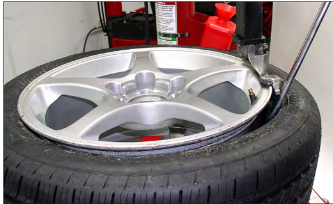
Figure 10 - Insert Bead Lifting Tool
