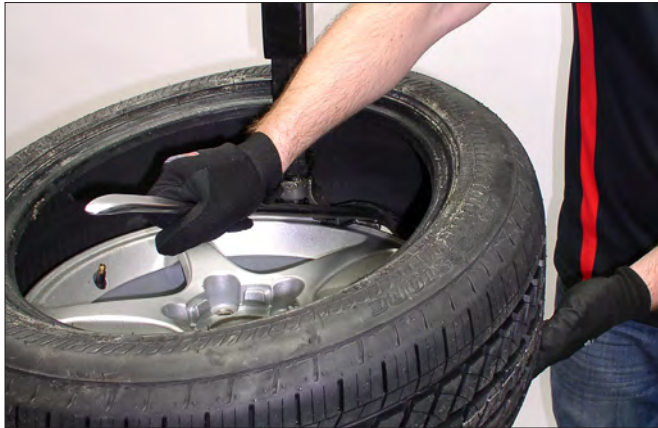
Figure 12 - Demounting Lower Bead
