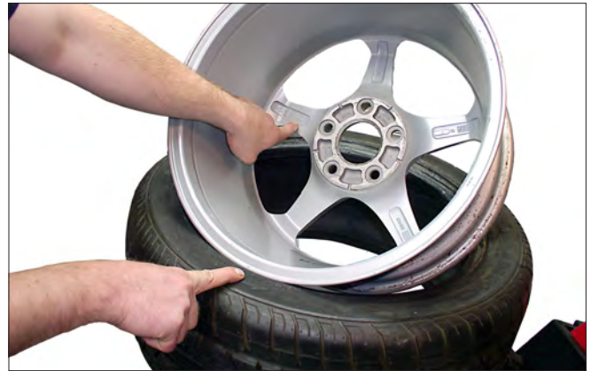
Figure 18 - Verify Size Match Between Tire and Wheel
