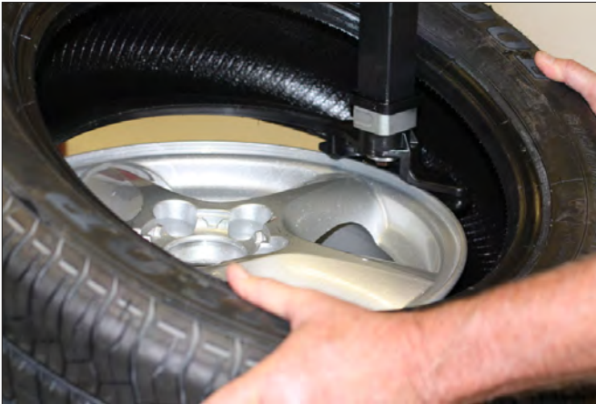
Figure 22 - Mounting Lower Bead
