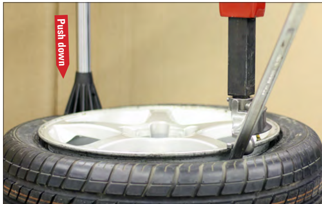
Figure 15 - Insert Bead Lifting Tool
