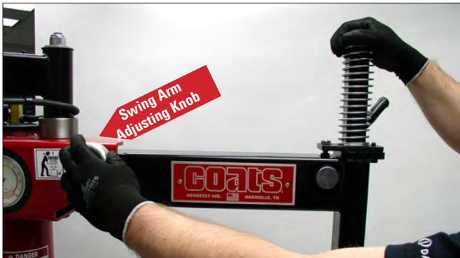
Figure 8 - Adjust Swing Arm to Position Tool Roller
