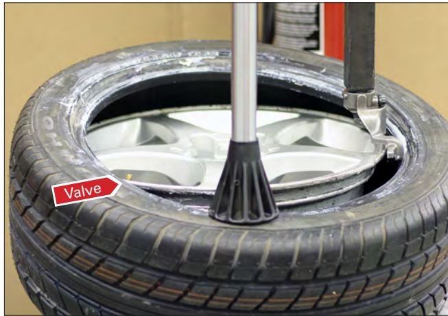
Figure 23 - Mount Top Bead Using Robo-Arm LR
