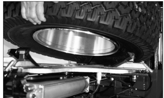
Figure 31B - Outside Clamped with Tire Removed
