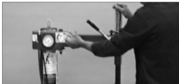
Figure 7 - Adjust Swing Arm to Position Head Roller
