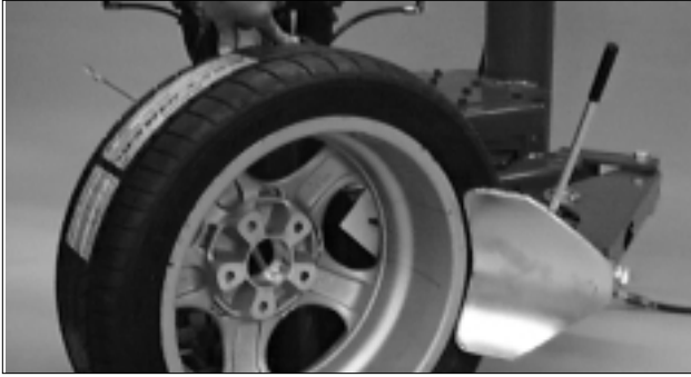
Figure 20 - Loosen Bottom Bead
