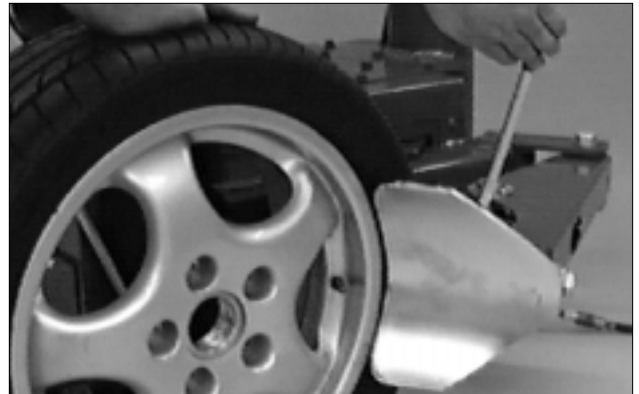
Figure 17 - Position Tire for Bead Loosening
