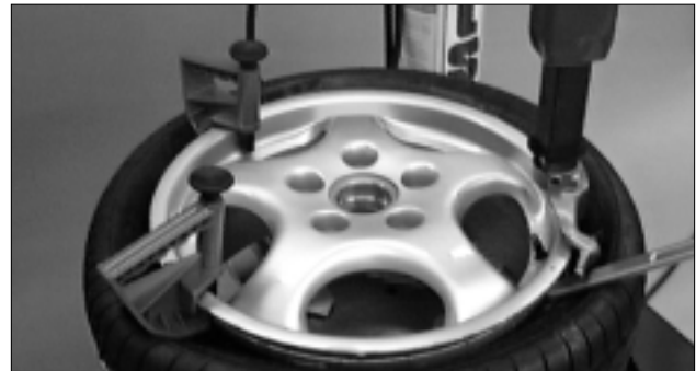
Figure 24 - Insert Bead Lifting Tool (Optional Drop Center Tools Shown)
