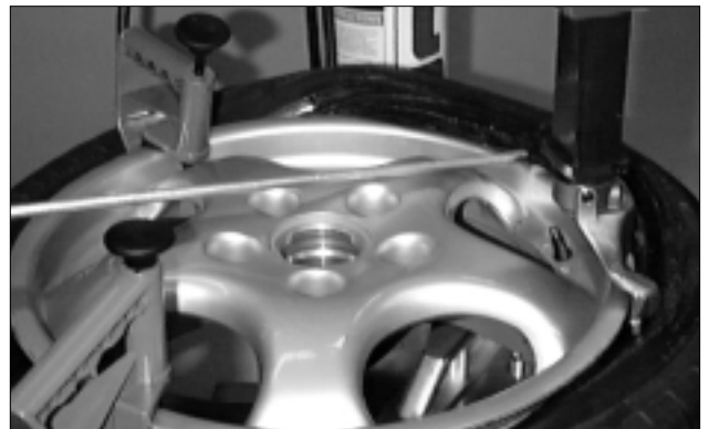
Figure 31 - Use Hooked End of Bead Lifting Tool
