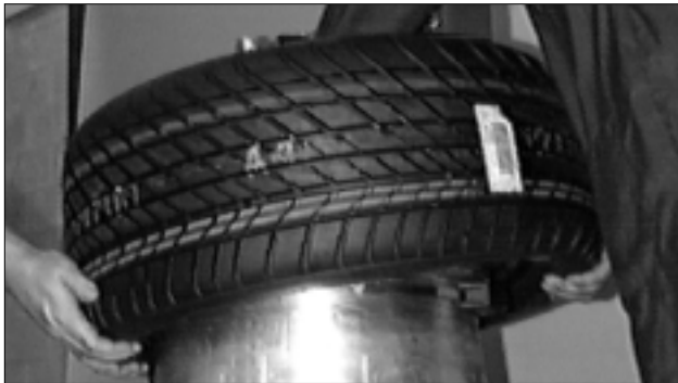
Figure 27 - Use Help on Lower Bead, Watch Sensor
