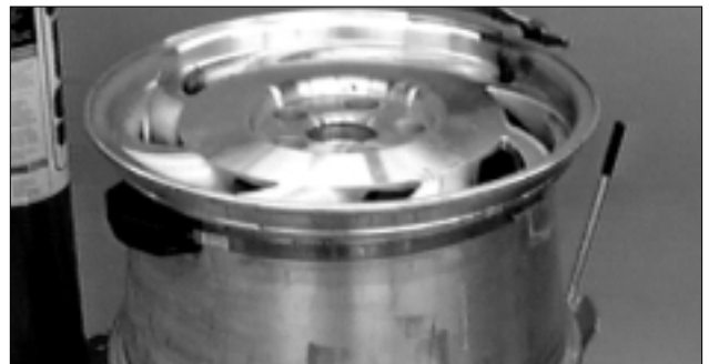
Figure 19- Wheel with Low Pressure Sensor/Transmitter
