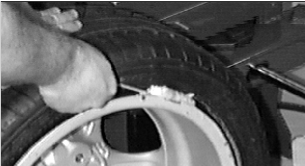
Figure 21 - Lubricate Bottom Bead
