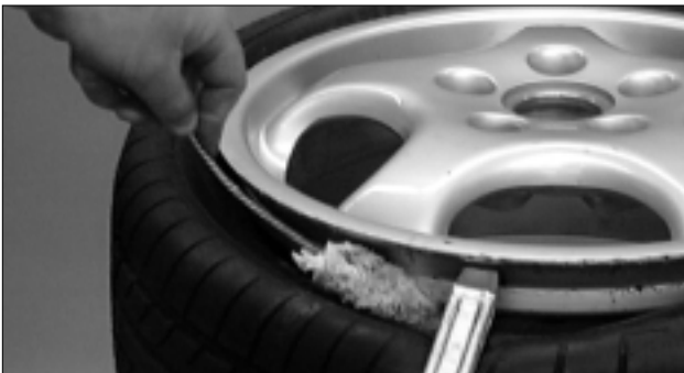
Figure 22 - Lubricate Upper Bead
