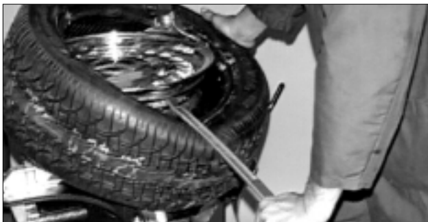
Figure 28 - Mount Lower Bead, Use Lifting Tool
