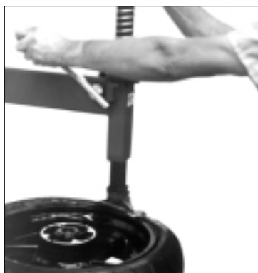
Figure 6 - Position Mount/Demount Tool
