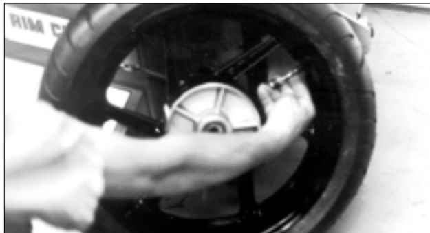
Figure 1 - Remove Valve Core to Deflate Tire
