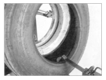
**1.** With the first bead removed, hook the roller tool over the outer bead and move the tool away from the rim to spread the beads and gain access to the inside of the tire.
