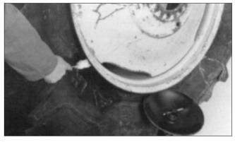
**3.** Rotate the wheel and slowly move the bead loosening disc into the sidewall until the bead is loosened.
