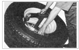
**4.** Lubricate tire beads and rim flange thoroughly: It may be easier to lubricate the top bead by letting the mount/demount tool push down on the bead and then rotating the tool with the lube swab following the tool. Demount the top bead in the usual manner). See section one.
