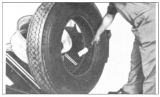
**3.** Lubricate Tire Beads: After inspecting tire thoroughly, lubricate both beads inside and out with an approved lubricant.
