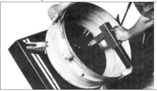
**2.** Lubricate Rim: After inspecting rim, thoroughly lubricate both bead seats with approved tire lubricant.
