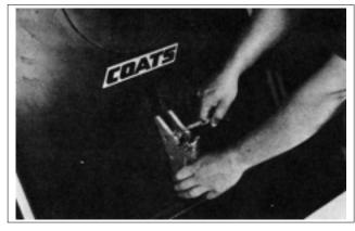
**2.** Clamp Adjustment: Adjust all three clamps to the proper wheel diameter range. The front hole position is for 19.5" to 24.5". The rear hole position is for 16" to 19.5".
