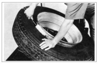
**5.** Lubricate both beads thoroughly: Both beads and the rim flange should be thoroughly lubricated with an approved tire lubricant before attempting to demount the tire. It may be easier to lubricate the bottom bead while the tire is in the bead loosener.
