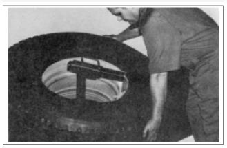
**2.** Position Top Bead: Manipulate and position the tire so that the bottom bead slips down toward its bead seat and the top bead rests evenly around the upper rim flange.
