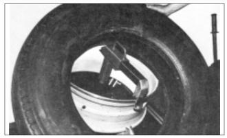
**4.** Position Tire: Lower table to a comfortable angle and rotate tool to approximately the 7 o'clock position. Lean tire over the rim and hook lower bead on mount/demount tool handle.
