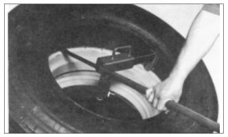
**4.** Demount Bottom Bead: Return mount/demount tool to the 12 o'clock position and insert bead lifter under bottom bead to the left of head. Again, make sure the opposite side of the bottom bead goes into drop center. Lift bottom bead over tool blade. Hold the bead lifter mount/demount tool clockwise and demounting bead. Make sure tool does not rotate into bead lifter during the operation.
