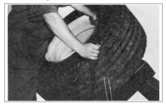
**3.** Clamping: Due to the stiff sidewall, it may be necessary to push down on the rim at the top as the clamps are being closed, to engage the rim. Lowering the table slightly will let the wheel's weight help in clamping.
