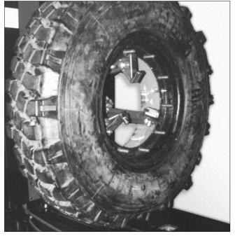
**12.** Move the carriage inward to position the wheel with the jaws in the center. Expand the arms so that the outer notch in the jaws clamp onto the inner rim of the wheel.
