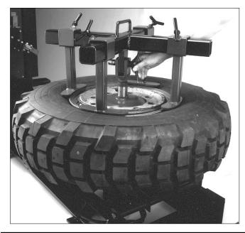
**4.** When the table is in the vertical position, manually center the tire and rim so that it lies perpendicular to the table cylinder.
