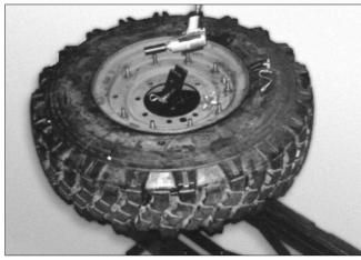
**6.** Remove the pressure sensor tubing. Remove the wheel nuts.
