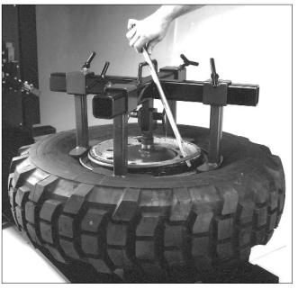
**6.** Compress the retaining ring and tire down enough to clear the lock ring. Using the ring tool, remove the lock ring.
