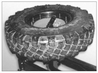
**9.** Remove the tire compressor and upper rim section.
