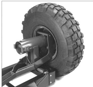
**2.** Place the tire and rim over the table top by rolling into place and then leaning back onto the table.
