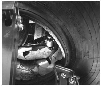
**12.** When inner tire is inside outer tire, use release rod by hooking over release bar on strap clamp as shown above.
