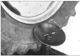
**2.** After locking the wheel on the chuck, move the bead loosening disc into position near the edge of the rim.
