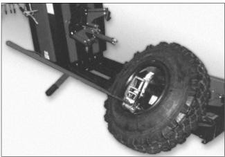
**14.** Lay the tire and insert on the floor with the strap buckle facing up and use the long tire bar to release the lock on the strap.
