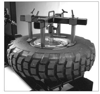
**25.** Press retaining ring down on rim seal and outer tire bead down below lock ring groove.
