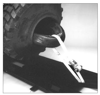
**16.** Move the carriage to the extended position, thus pulling the inner tire out of the outer tire. If the two tires are not separated when the carriage has reached its extended position, further travel can be reached by raising the vertical cylinder until the two tires are separated.
