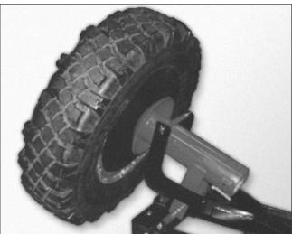
**5.** With another person holding the wheel in place, move the carriage in, bringing the end plate and wheel up into a horizontal position.
