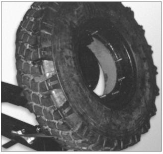
**22.** Remove the tire and rim assembly from the tire changer's jaws and then move the wheel to the end of the machine.
