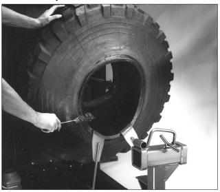
**8.** Place the two bead spreaders into the lower edge of the bead with the other end hooked into the openings of the tire ramps (angles welded to the side rails). Then, lift the tire up until the bead is spread open slightly.
