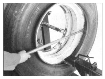
**5.** Pry the bead out over the rim. *Note:* You may have to assist the bead opposite the tool into the drop center. Use one of the tire tools to pry the top bead into the drop center.
