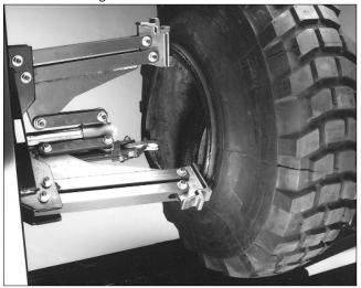
**7.** Roll the outer tire onto the carriage and clamp the bead into the deepest "V" in jaws.
