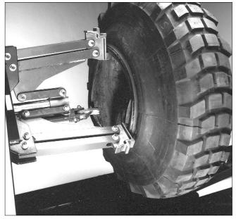
**14.** Roll tire onto carriage platform and clamp bead into deepest "V" in jaws.
