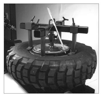
**26.** Install lock ring and insure that it is down properly in lock ring groove.
