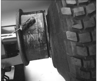
**17.** Place rim over table top and tire over cylinder shaft. Apply liberal amount of tire lube to rim as shown above.
