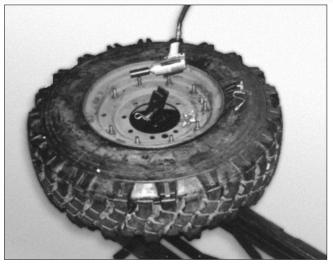
**29**. Draw the sections together using a cross pattern on the wheel bolts. Torque to wheel manufacturer's specifications.
