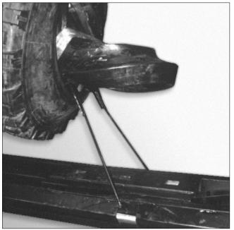
**7.** Lift the run flat insert and put one end in the tire far enough for the buckle to be beyond the bead of the tire. Rotate the insert until the buckle is facing down. **Note:** the larger end of the insert should be in the tire and at the top.
