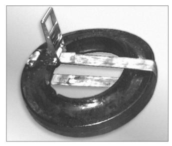
**4.** On the floor spread out the 4 inch wide strap with the buckle facing down. Lay the run flat insert on the strap as close to the buckle as possible and with one of the three relief grooves lined up on the strap. Bring the long end of the strap over the insert and install it in the buckle.
