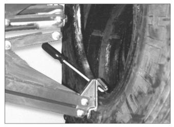
**19.** Raise the tire and rotate until a second jaw has hooked the bead.
