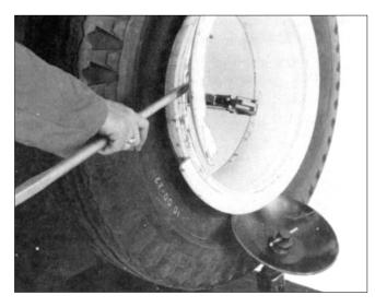
**3.** Use the ring tool to remove the lock ring(s).
