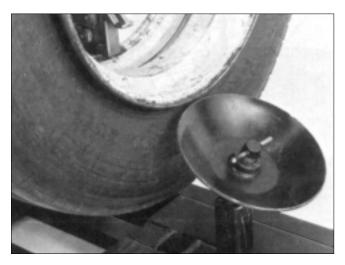
**2.** Position the bead loosening disc in one of the square holes in the carriage closest to the outer edge of the tire.
