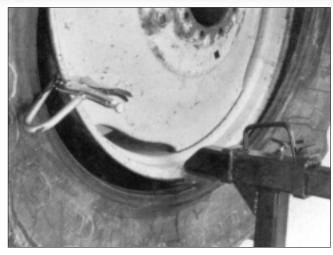
**3.** Move the combo tool into position near the edge of the rim.
