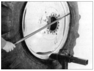
**3.** Rotate the wheel counterclockwise while maintaining pressure on the spade tool until the outer bead is demounted. Push the valve stem inside the rim and pull the inner tube out of the tire.
