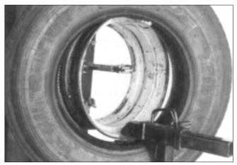
**4.** Securely clamp the vise grip to the rim edge at a position to the left of the combo tool. Rotate the chuck clockwise until the vise grip hooks the inner bead and lifts the tire.
