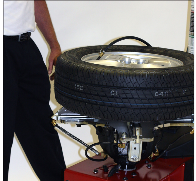
Figure 25 - Stand Back during Bead Seat
