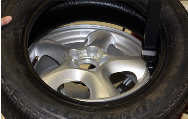
Figure 19 - Position Tire Against Mount/Demount Tool
