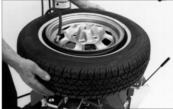
Figure 24 - Lift Tire Upwards for Bead Sealing
