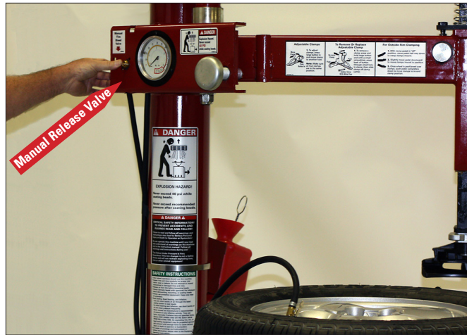
Figure 26 - Location of Manual Release Valve
