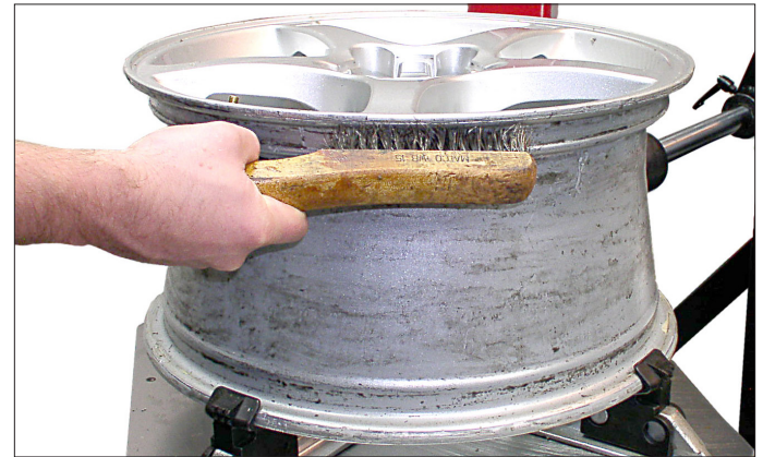
Figure 17 - Inspect and Clean the Wheel
