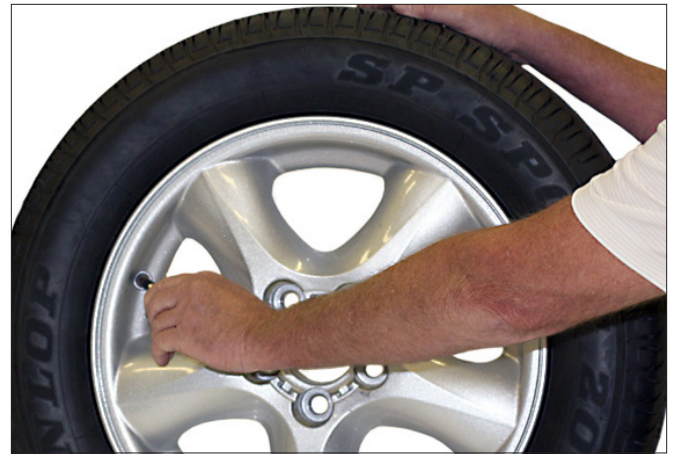
Figure 1 - Remove Valve Core to Deflate Tire
