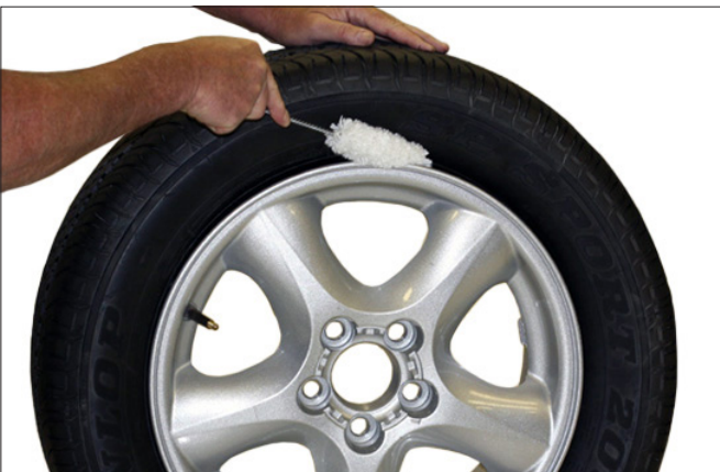
Figure 5 - Apply Rubber Lubricant to Tire Beads
