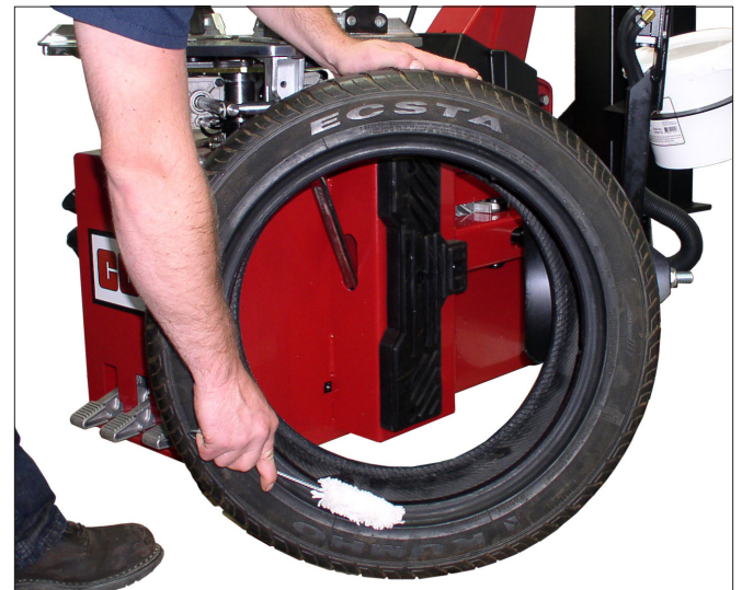
Figure 18 - Lubricate Tire Beads Liberally
