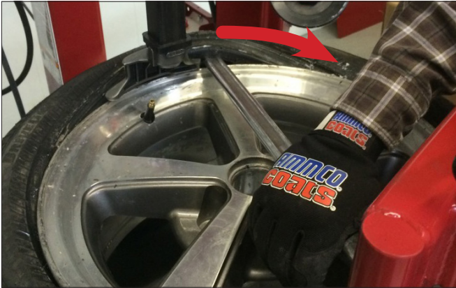
Figure 12 - Demount Upper Bead
