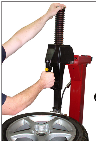
Figure 9 - Position Mount/Demount Tool
