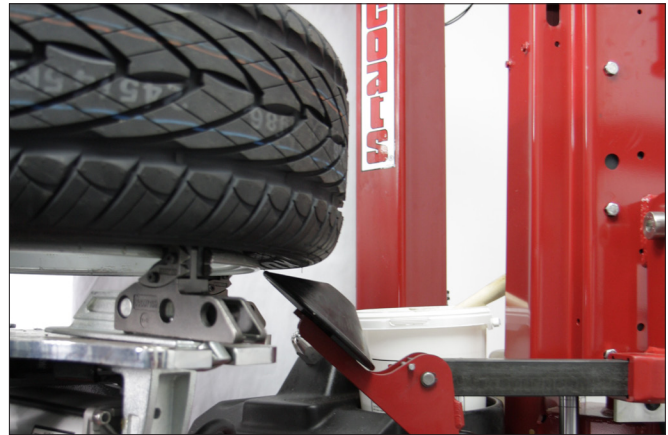
Figure 14 - Disk-assist Aiding Lower Bead Demount
