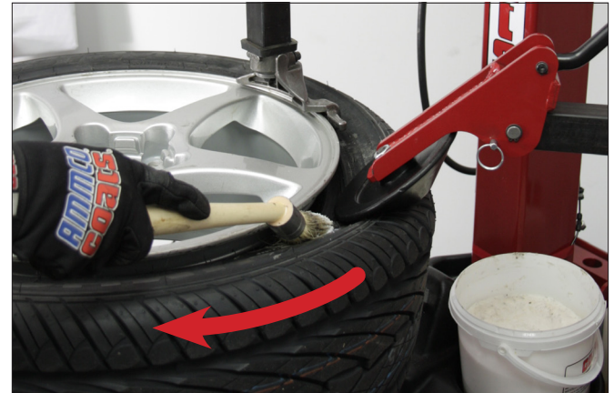
Figure 10 - Apply Rubber Lubricant to the Beads
