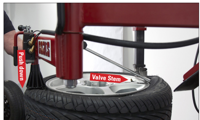
Figure 11 - Insert Bead Lifting Tool
