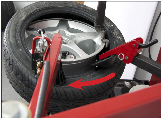
Fig 21 - Hold Tire Bead In Rim Drop Center
