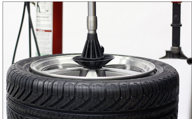
Figure 7 - Robo-Arm® Aids Clamping
