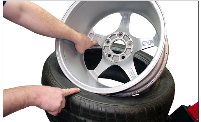
Figure 16 - Verify Size Match Between Tire and Wheel
