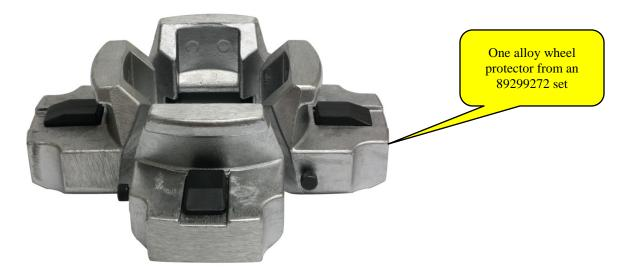
To prevent damaging the protectors, all four protectors must be removed before fully closing the clamps.
