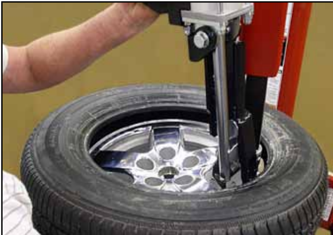
Figure 6 - Push Control Handle Up To Lift Bead Over Rim
