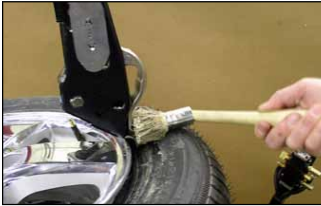
Figure 1 - Apply lubricant to Bead Lifter Tool
