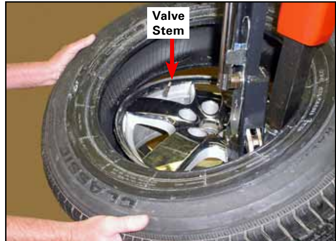
Figure 7 - Position Tire Against Bead Lifter Tool
