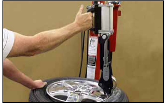
Figure 4 - Leverless Tool Hooked Under Tire Bead
