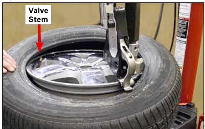
Figure 8 - Position Valve Stem In Front Of Bead Lock
