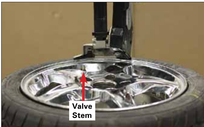
Figure 2 - Position Valve Stem By the Bead Lifter Tool
