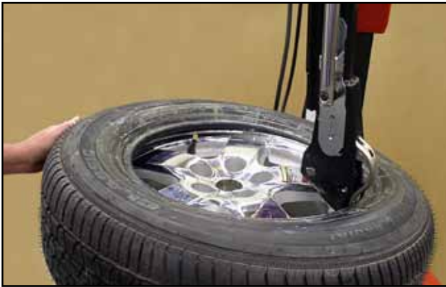
Figure 5 - Bead Lifter Tool Hooked Under Tire Bead
