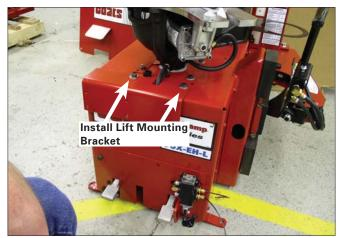
**12.** Install the wheel lift assembly to the lift mounting bracket using three thread cutting screws.
