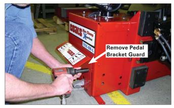
**5.** Remove the machine's side panel using a speed handle or drill and 3/8-inch socket.
