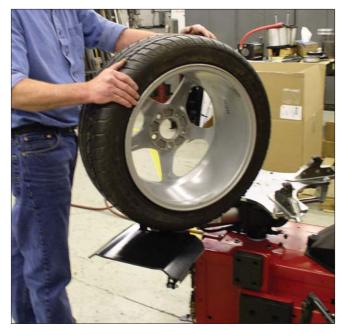
**4.** With the tire resting on the back of the clamp, lower it so that the rim fits in the clamps.
