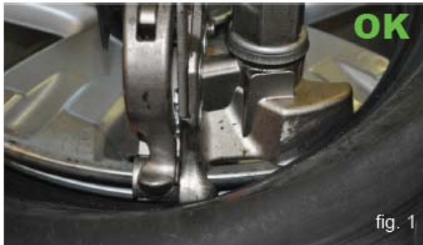
fig. 1 Bead correctly positioned over the left side of the mounting tool and under it on its right side.
