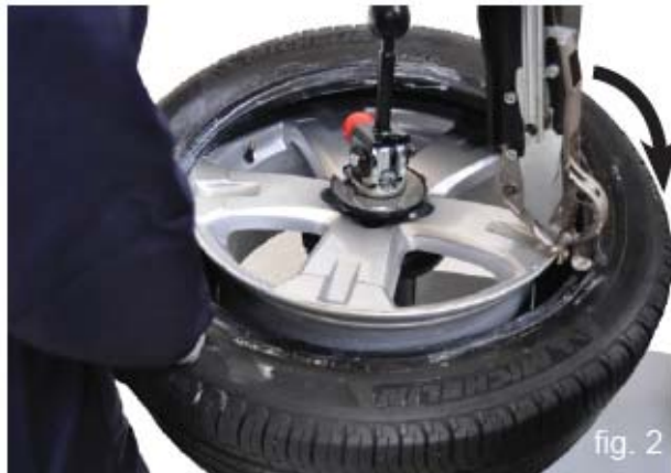
fig. 2 Press the pedal 2 to rotate the wheel clockwise, contemporarily press the tire manually from "5 o'clock" position to force the upper bead at drop-centre position. Keep it pressed while rotating up to "8 o'clock" position to complete the upper bead mounting (fig. 2).
