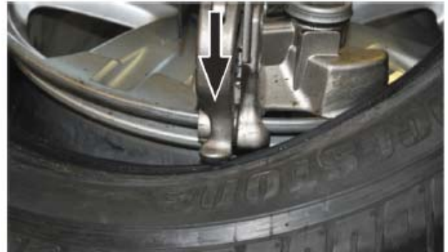
fig. 1 Bead correctly positioned over the left side of the mounting tool and under it on its right side, thus it can be slightly lowered for easy tire mounting.
