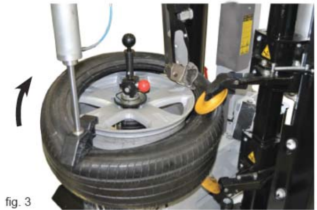
fig. 2 Press the pedal 2 to rotate the wheel clockwise, contemporarily press the tire manually from "5 o'clock" position to force the upper bead at drop-centre position. Keep it pressed while rotating up to "8 o'clock" position to complete the upper bead mounting (fig. 2).
