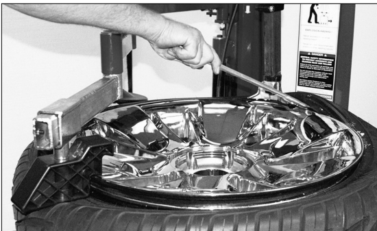
Figure 34 - Lift Bead Carefully onto Duckhead
