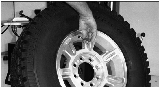
Figure 1 - Remove Valve Core to Deflate Tire
