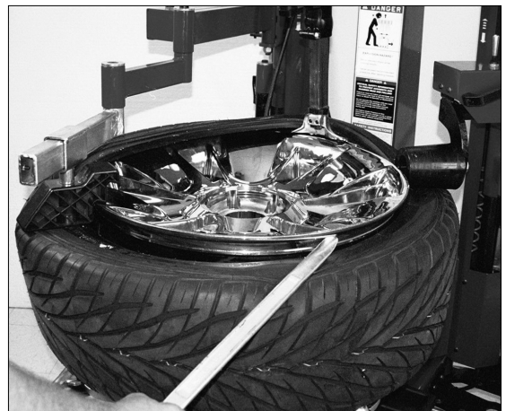
Figure 42 - Utilize the Lift Tool if Necessary
