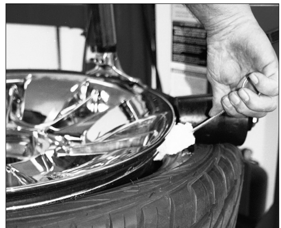
Figure 32 - Lubricate Upper Bead
