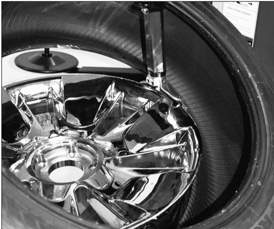
Figure 39 - Mount the Lower Bead
