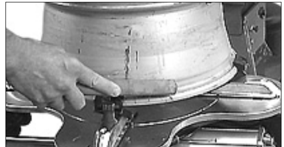
Figure 15 - Inspect and Clean the Wheel
