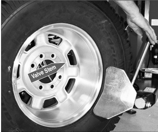
Figure 28 - Loosen Bottom Bead
