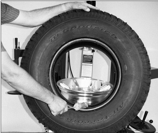
Figure 16 - Lubricate Tire Beads Liberally
