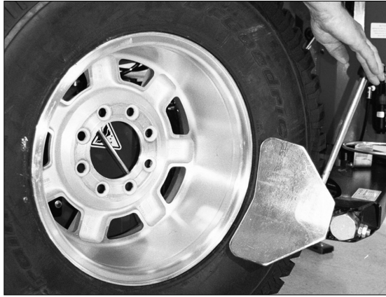
Figure 4 - Position Tire and Bead Loosener Shoe with Wheel Turned Around
