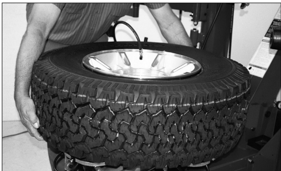
Figure 20 - Lift Tire Upwards for Bead Sealing
