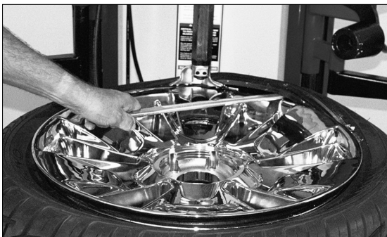
Figure 35 - Start Upper Bead Removal
