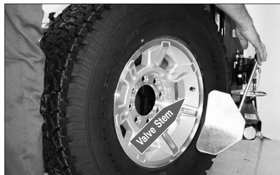
Figure 3 - Position Tire and Bead Loosener Shoe
