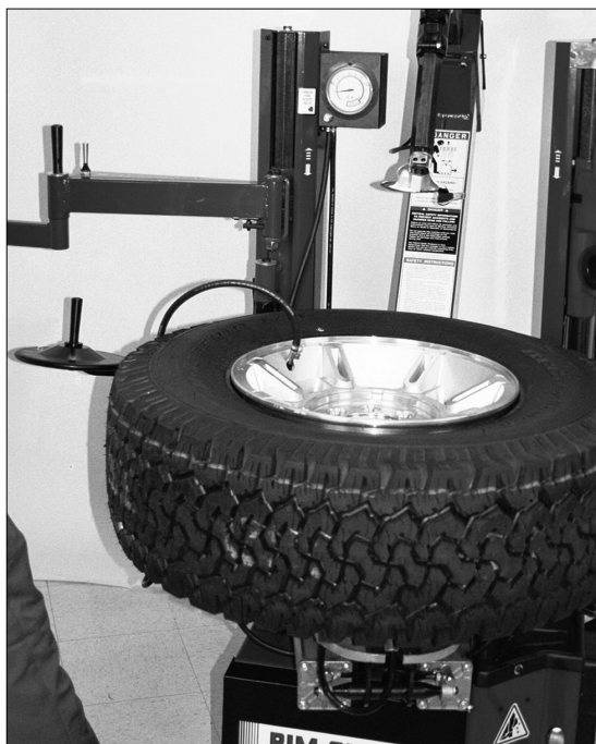
Figure 21 - Stand Back during Bead Seat
