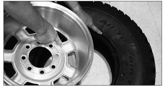
Figure 14 - Verify Size Match Between Tire and Wheel
