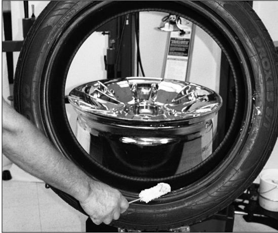
Figure 38 - Lubricate Tire Beads
