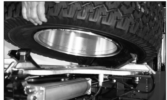
Figure 31B - Outside Clamped with Tire Removed
