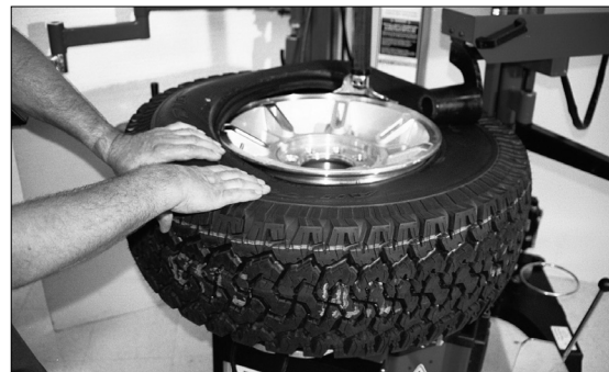
Figure 19 - Mounting Top Bead
