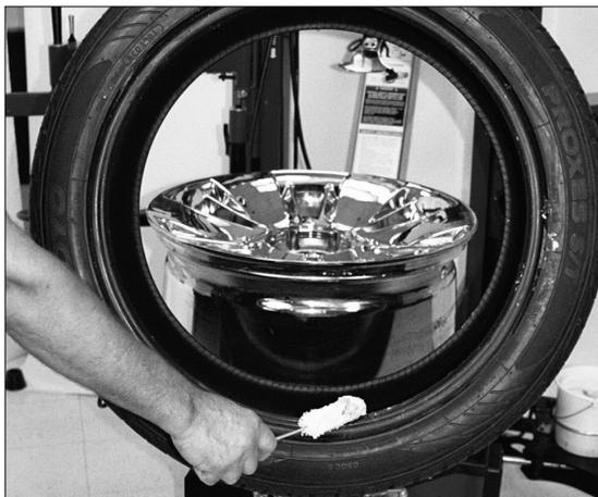
Figure 38 – Lubrification des talons
