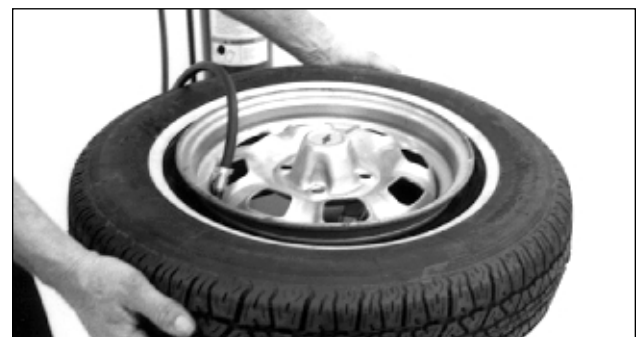
Figure 18 - Lift Tire Upwards for Bead Sealing
