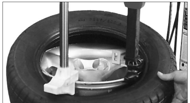
Figure 33 - Mount Upper Bead, Use Helper
