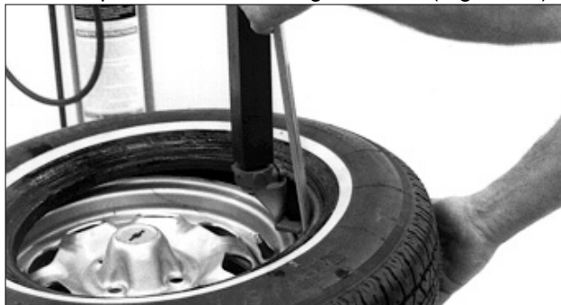
Figure 12 - Demounting Lower Bead
