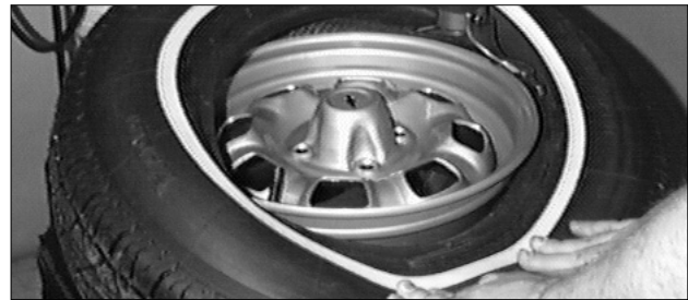
Figure 17 - Mounting Top Bead
