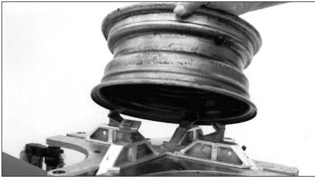
Figure 5 – Place Tire/Wheel Assembly on Table Top
