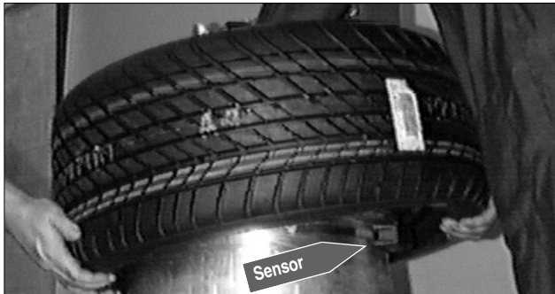
Figure 31 - Sensor/ Transmitter Location
