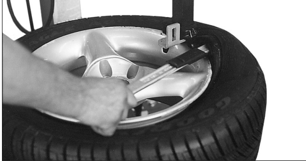
Figure 30 - Holding Lifting Tool in Place and Rotate Wheel
