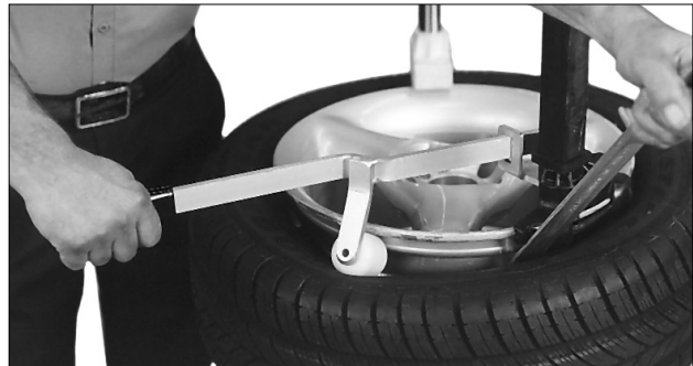
Figure 28 - Insert Bead Lifting Tool
