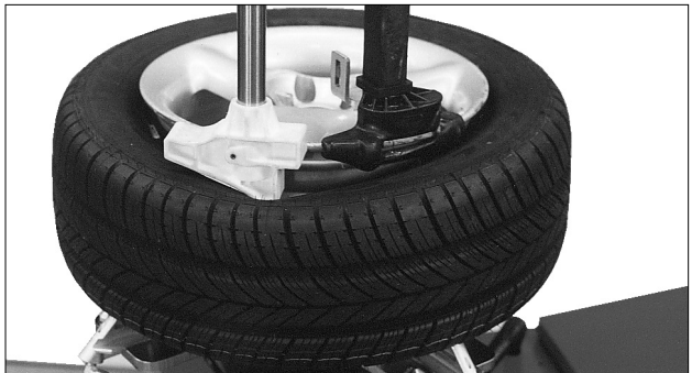
Figure 25 - Helper Foot Depressing Sidewall of Tire
