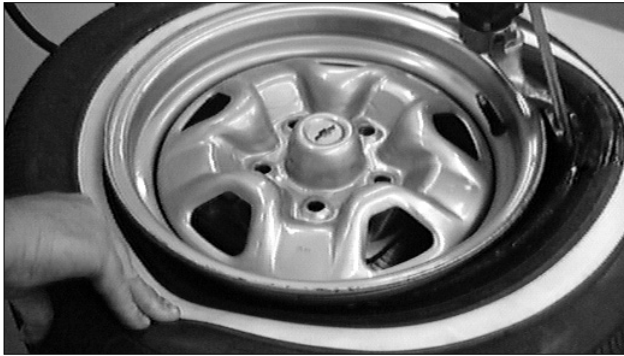
Figure 10 - Insert Bead Lifting Tool
