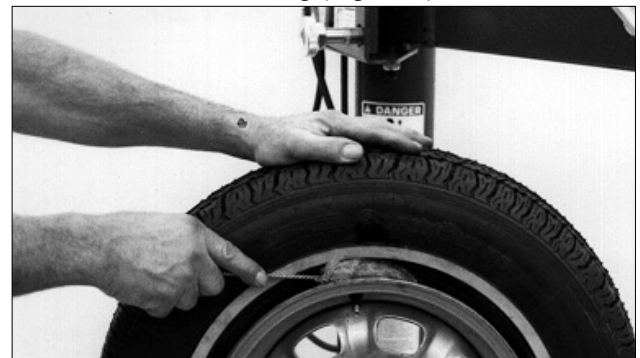
Figure 3 – Apply Rubber Lubricant to Tire Beads
