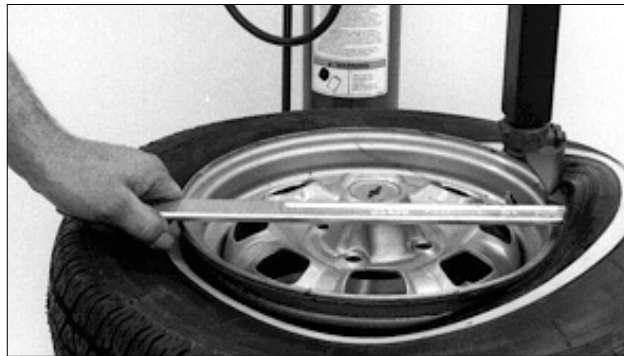
Figure 11 - Lift Bead Over Demount Head
