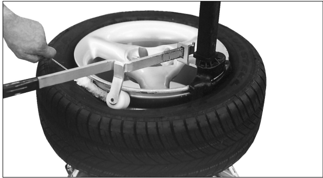
Figure 26 - Lubricate Upper Bead
