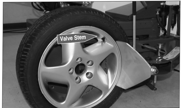
Figure 2 – Position Tire and Bead Loosener Shoe
