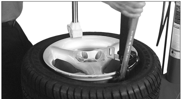
Figure 29 - Rotate Lifting Tool Down for Demount
