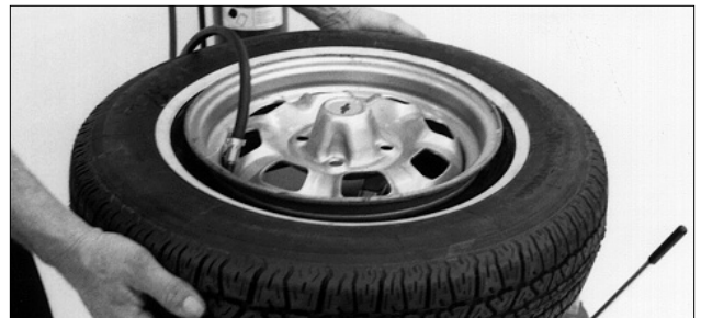
Figure 18 - Lift Tire Upwards for Bead Sealing
