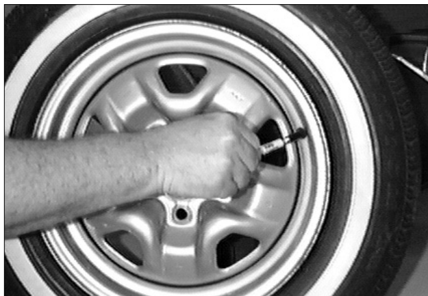
Figure 1 – Remove Valve Core to Deflate Tire
