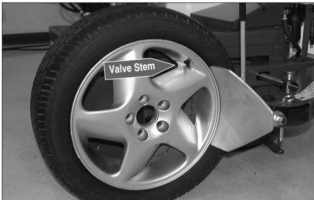
Figure 20 - Position Tire for Bead Loosening
