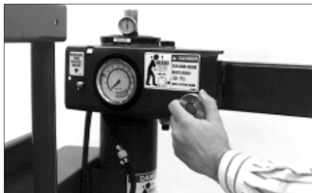
Figure 7 - Adjust Swing Arm to Position Head Roller
