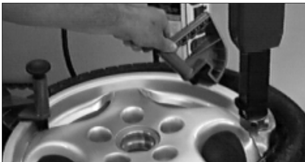
Figure 30 - Remove Drop Center Tools Before Tool Head
