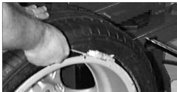
Figure 25 - Lubricate Bottom Bead
