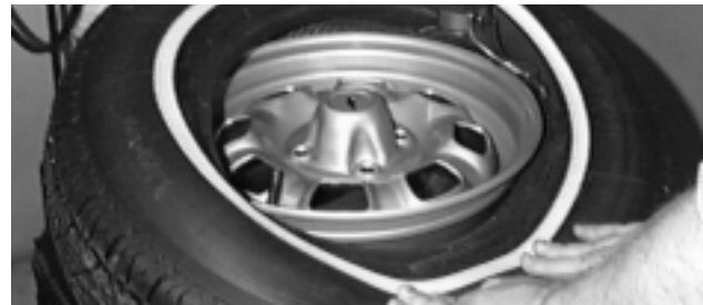
Figure 16 - Mounting Top Bead
