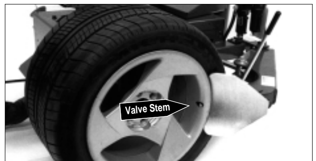
Figure 21 - Position Tire for Bead Loosening and Place Positioning Pin in Proper Location for Wide Wheels
