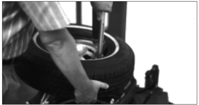
Figure 11 - Demounting Lower Bead
