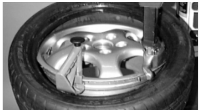
Figure 33 - Mounting Top Bead
