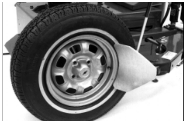
Figure 2 – Position Tire and Bead Loosener Shoe
