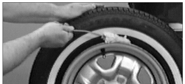
Figure 3 – Apply Rubber Lubricant to Tire Beads
