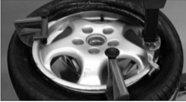
Figure 34- Add Second Drop Center Tool
