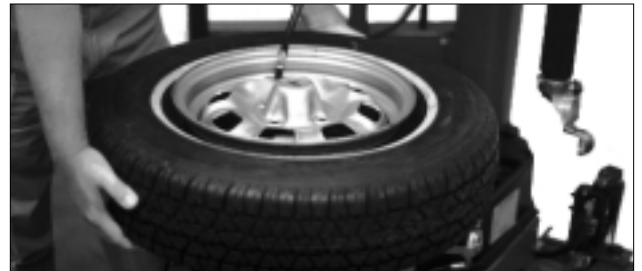
Figure 17 - Lift Tire Upwards for Bead Sealing
