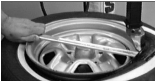
Figure 10 - Lift Bead Over Demount Head
