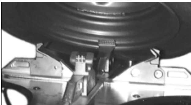
Figure 5 – Place Tire/Wheel Assembly on Table Top
