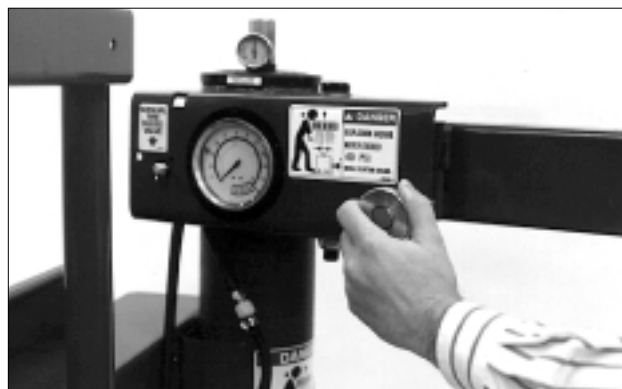
Figure 7 - Adjust Swing Arm to Position Head Roller
