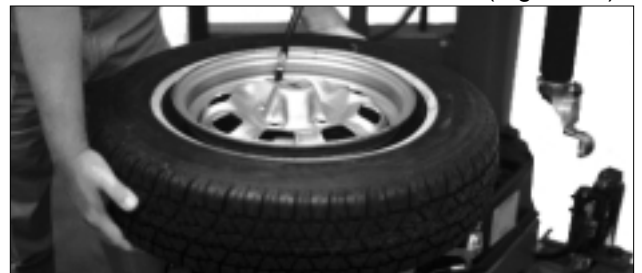
Figure 17 - Lift Tire Upwards for Bead Sealing
