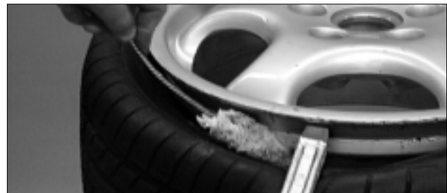
Figure 26 - Lubricate Upper Bead
