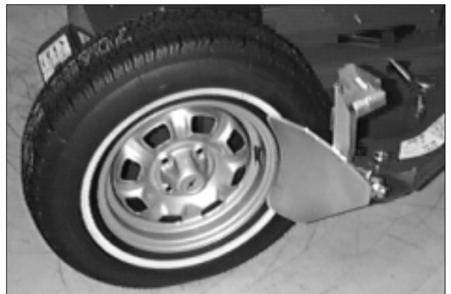
Figure 2 – Position Tire and Bead Loosener Shoe
