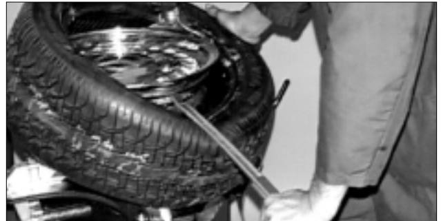
Figure 32 - Mount Upper Bead, Use Lifting Tool
