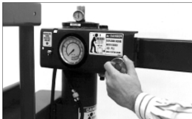
Figure 7 - Adjust Swing Arm to Position Head Roller
