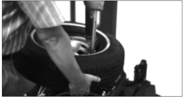
Figure 11 - Demounting Lower Bead
