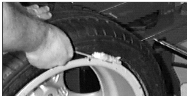
Figure 25 - Lubricate Bottom Bead
