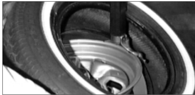
Figure 15 - Position Tire Against Mount/Demount Head
