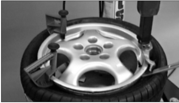
Figure 28 - Insert Bead Lifting Tool (Optional Drop Center Tools Shown)
