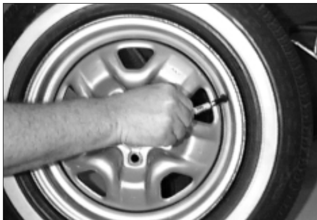
Figure 1 – Remove Valve Core to Deflate Tire
