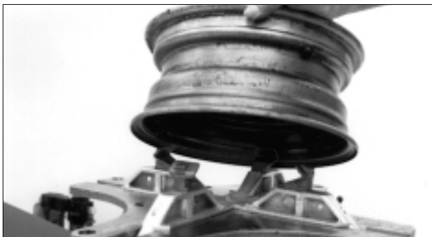
Figure 5 – Place Tire/Wheel Assembly on Table Top
