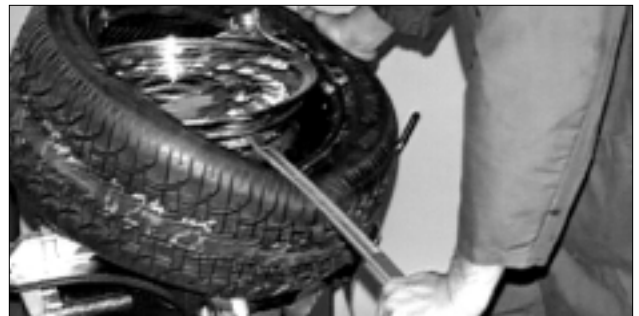
Figure 32 - Mount Upper Bead, Use Lifting Tool
