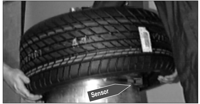
Figure 31 - Use Help on Lower Bead, Watch Sensor
