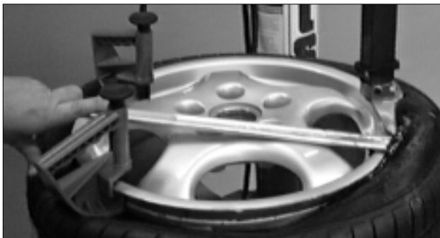
Figure 29 - Pull Lifting Tool Down and Rotate Wheel
