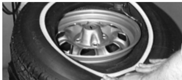
Figure 16 - Mounting Top Bead
