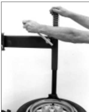
Figure 6 - Position Mount/Demount Tool
