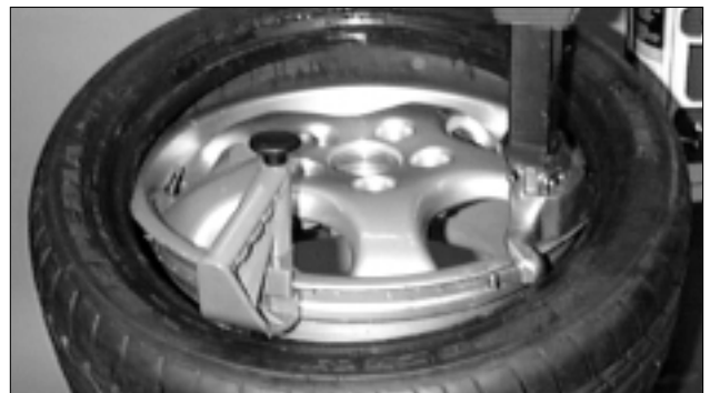
Figure 33 - Mounting Top Bead
