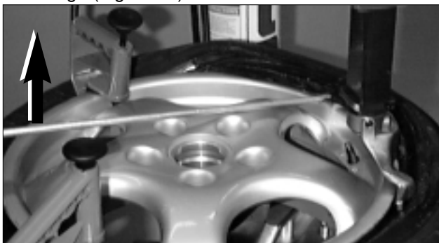
Figure 35 - Use Hooked End of Bead Lifting Tool
