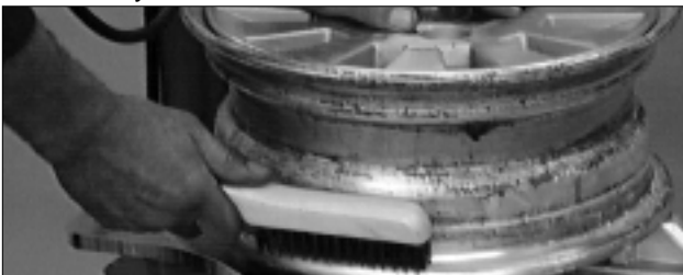
Figure 13 - Inspect and Clean the Wheel
