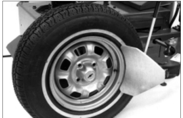
Figure 2 – Position Tire and Bead Loosener Shoe
