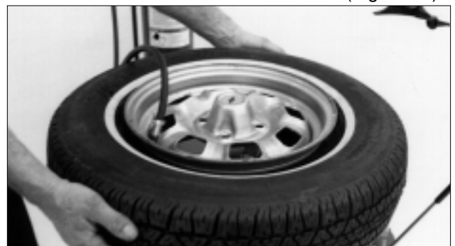
Figure 17 - Lift Tire Upwards for Bead Sealing
