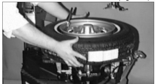
Figure 17 - Lift Tire Upwards for Bead Sealing
