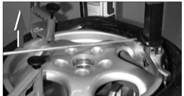
Figure 34 - Use Hooked End of Bead Lifting Tool
