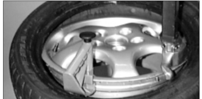
Figure 32 - Mounting Top Bead
