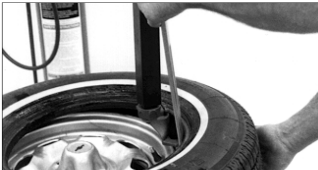
Figure 11 - Demounting Lower Bead
