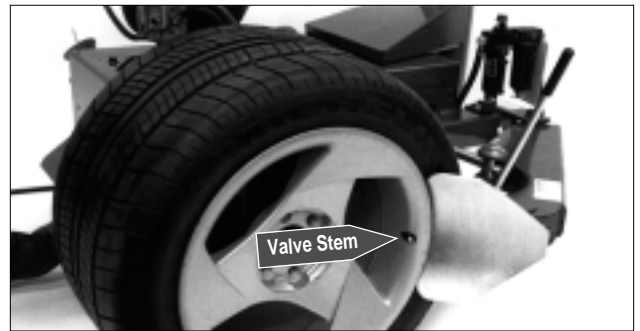
Figure 20 - Position Tire for Bead Loosening
