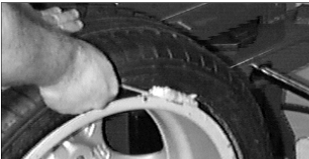
Figure 24 - Lubricate Bottom Bead
