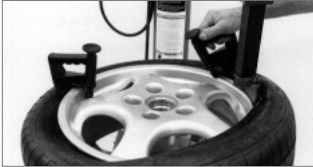
Figure 29 - Remove Drop Center Tools Before Tool Head
