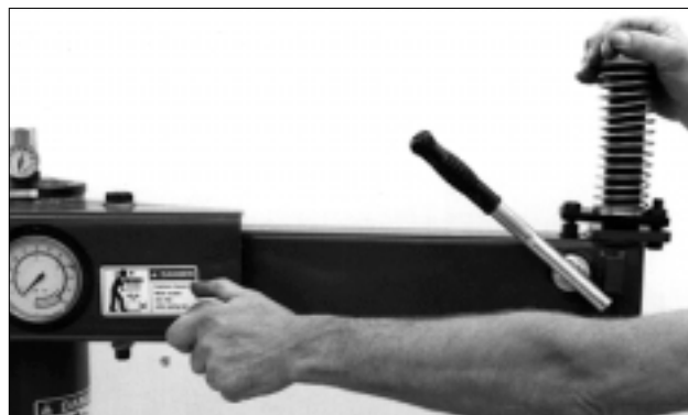
Figure 7 - Adjust Swing Arm to Position Head Roller
