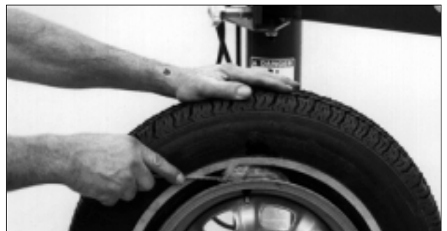
Figure 3 – Apply Rubber Lubricant to Tire Beads
