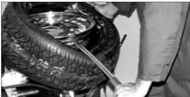
Figure 31 - Mount Upper Bead, Use Lifting Tool
