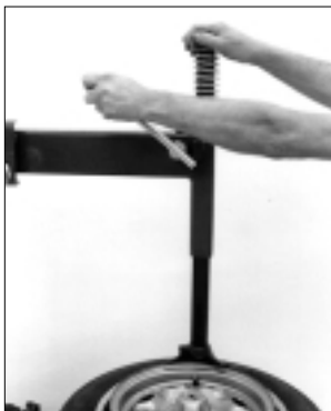
Figure 6 - Position Mount/Demount Tool
