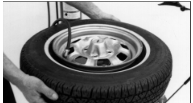
Figure 17 - Lift Tire Upwards for Bead Sealing
