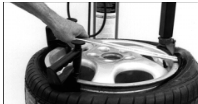
Figure 28 - Pull Lifting Tool Down and Rotate Wheel
