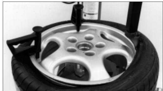
Figure 27 - Insert Bead Lifting Tool (Optional Drop Center Tools Shown)
