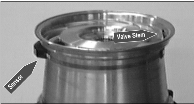
Figure 22 - Wheel with Low Pressure Sensor/Transmitter
