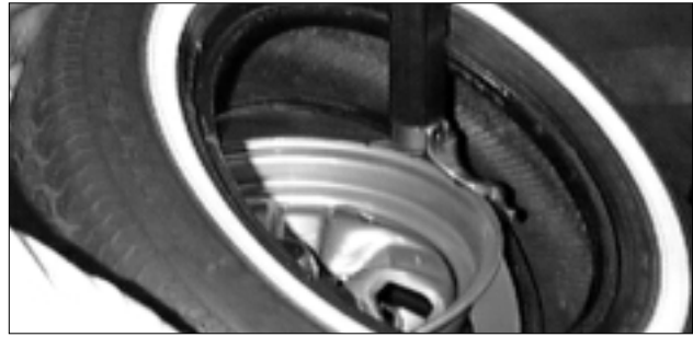
Figure 15 - Position Tire Against Mount/Demount Head
