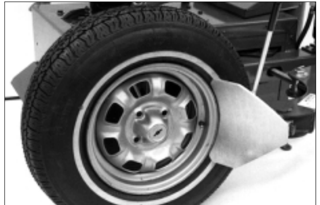
Figure 2 – Position Tire and Bead Loosener Shoe
