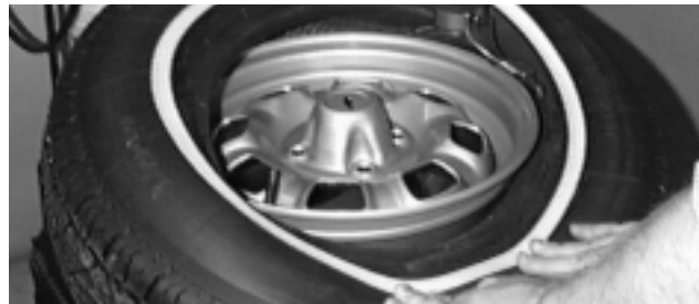
Figure 16 - Mounting Top Bead
