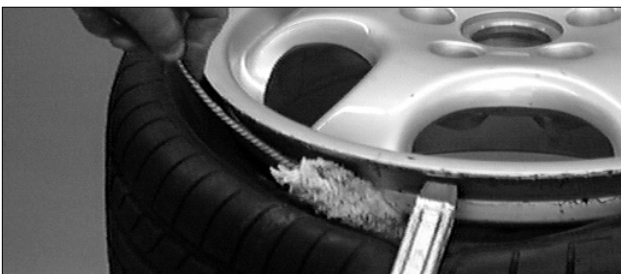
Figure 26 - Position Valve Stem Under Demount Head
