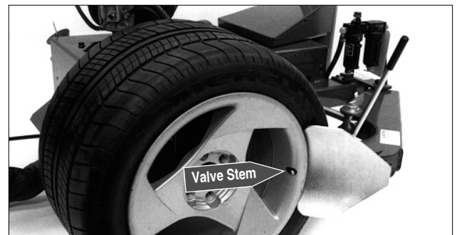
Figure 20 - Position Tire for Bead Loosening
