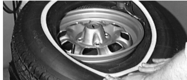
Figure 15 - Position Tire Against Mount/Demount Head
