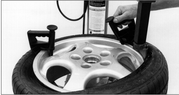
bead demount procedure (Figure 30).
