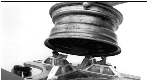
Figure 5 – Place Tire/Wheel Assembly on Table Top
