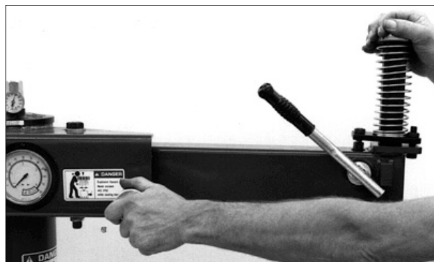
Figure 7 - Adjust Swing Arm to Position Head Roller
