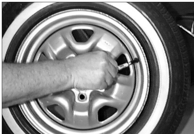
Figure 1 – Remove Valve Core to Deflate Tire
