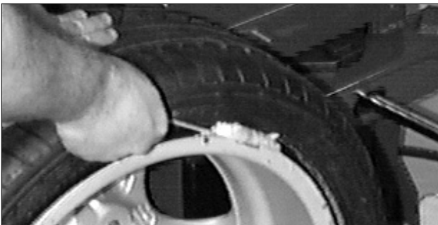
Figure 25 - Lubricate Upper Bead
