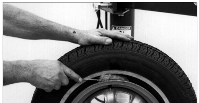
Figure 3 – Apply Rubber Lubricant to Tire Beads
