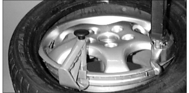
Figure 32 - Mounting Top Bead
