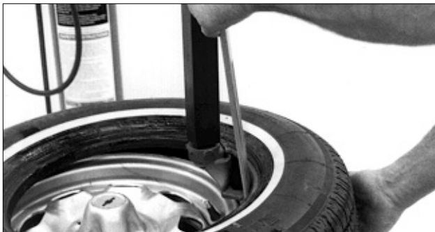
Figure 11 - Demounting Lower Bead
