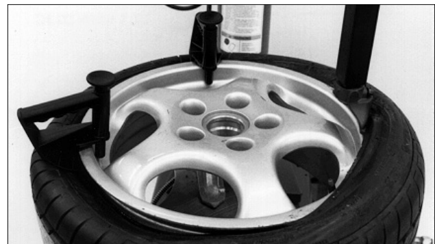
Figure 28 - Pull Lifting Tool Down and Rotate Wheel
