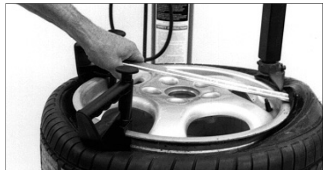
Figure 29 - Remove Drop Center Tools Before Tool Head
