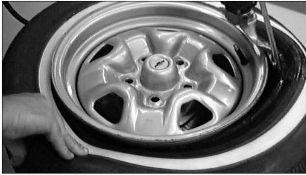
Figure 9 - Insert Bead Lifting Tool
