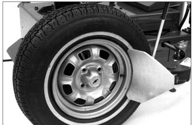
Figure 2 – Position Tire and Bead Loosener Shoe
