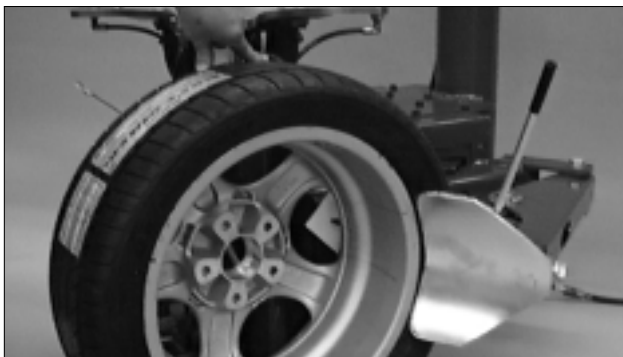
Figure 21 - Loosen Bottom Bead
