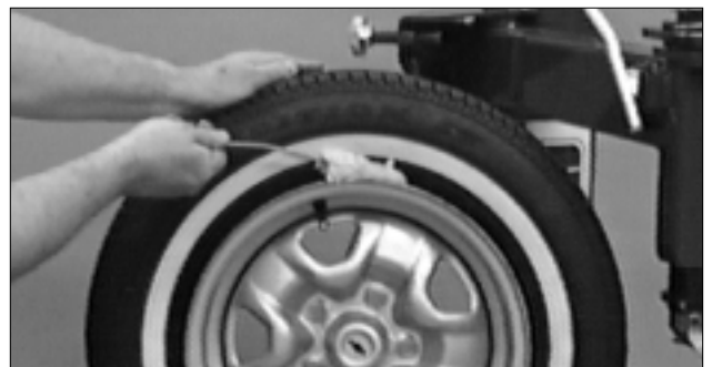
Figure 3 - Apply Rubber Lubricant to Tire Beads
