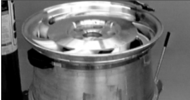
Figure 20 - Wheel with Low Pressure Sensor/Transmitter
