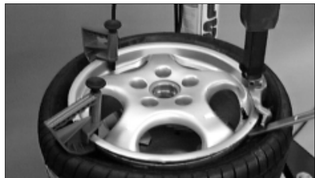
Figure 25 - Insert Bead Lifting Tool (Optional Drop Center Tools Shown)
