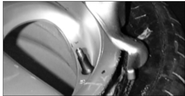
Figure 24 - Position Valve Stem Under Demount Head
