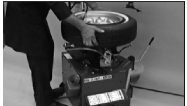
Figure 15 - Lift Tire Upwards for Bead Sealing
