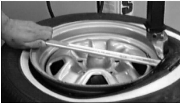
Figure 10 - Lift Bead Over Demount Head
