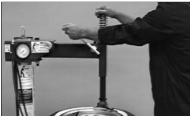
Figure 6 - Position Mount/Demount Tool
