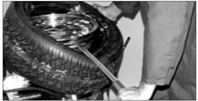
Figure 29 - Mount Lower Bead, Use Lifting Tool
