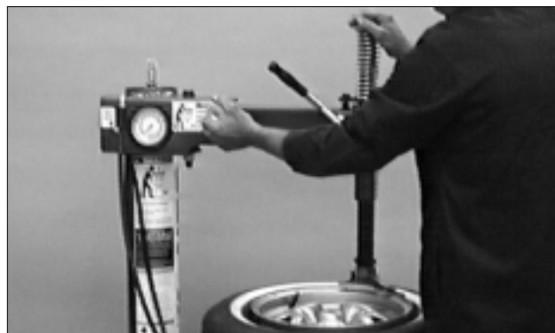
Figure 7 - Adjust Swing Arm to Position Head Roller
