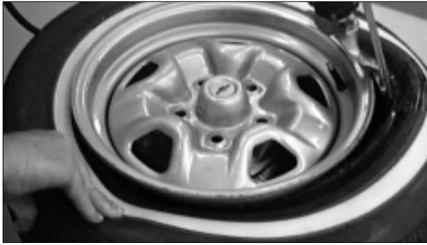
Figure 9 - Insert Bead Lifting Tool
