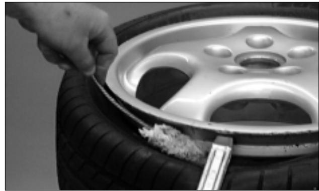
Figure 23 - Lubricate Upper Bead
