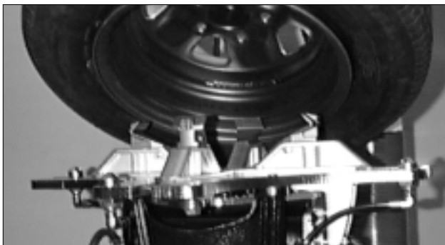
Figure 5 - Place Tire/Wheel Assembly on Table Top
