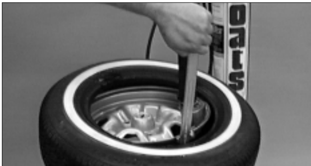
Figure 11 - Demounting Lower Bead
