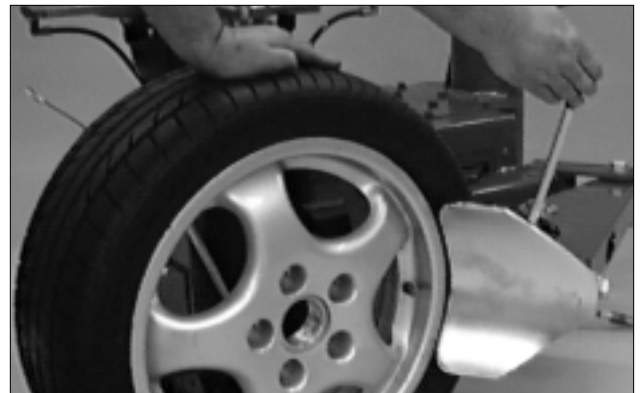
Figure 18 - Position Tire for Bead Loosening
