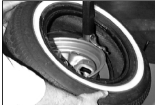
Figure 14 - Position Tire Against Mount/Demount Head
