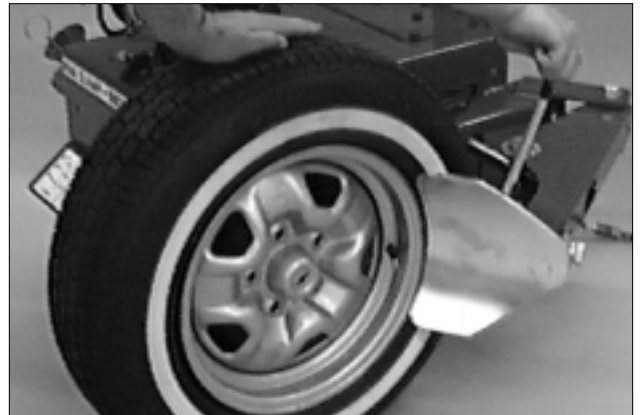
Figure 2 - Position Tire and Bead Loosener Shoe
