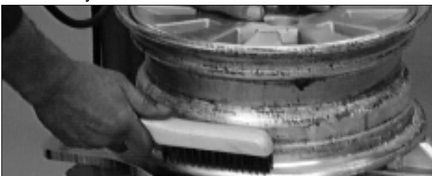
Figure 12 - Inspect and Clean the Wheel
