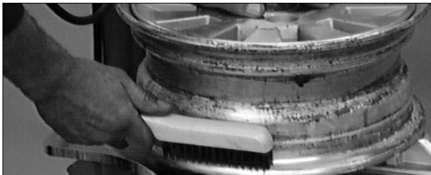
Figure 12 - Inspect and Clean the Wheel
