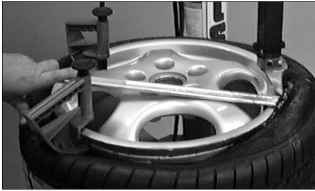
Figure 26 - Pull Lifting Tool Down and Rotate Wheel
