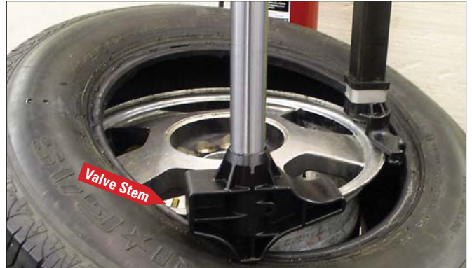
Fig 23 - Use Robo Arm To Hold Tire In Rim Drop Center
