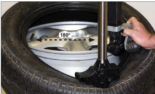
Figure 21 - Position Valve Stem 180° Ahead of Mount Tool
