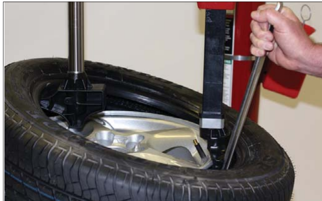
Figure 41 - Rotate Lifting Tool Down for Demount
