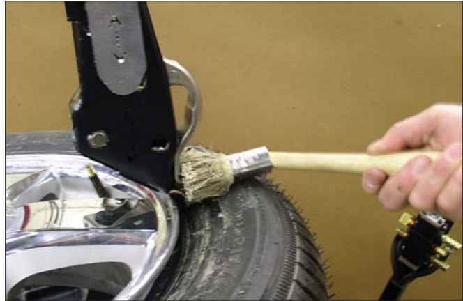
Figure 49 - Apply Lubricant to Bead Lifter Tool Hook
