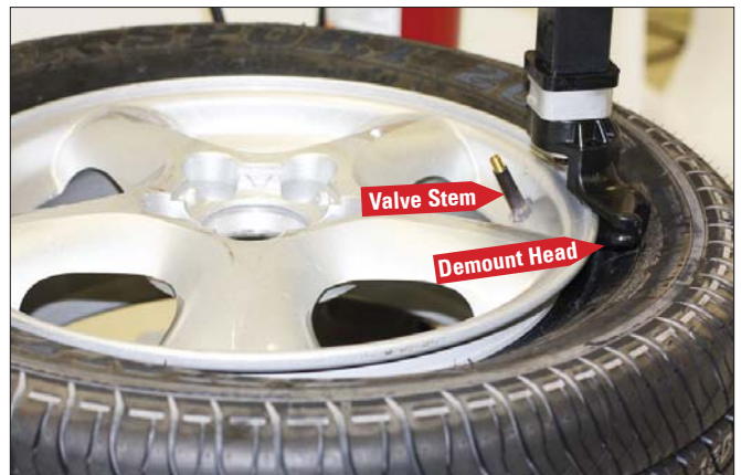
Figure 36 - Position Valve Stem Under Demount Tool
