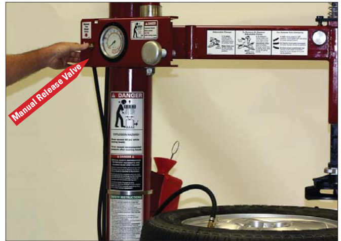
Figure 27 - Location of Manual Release Valve
