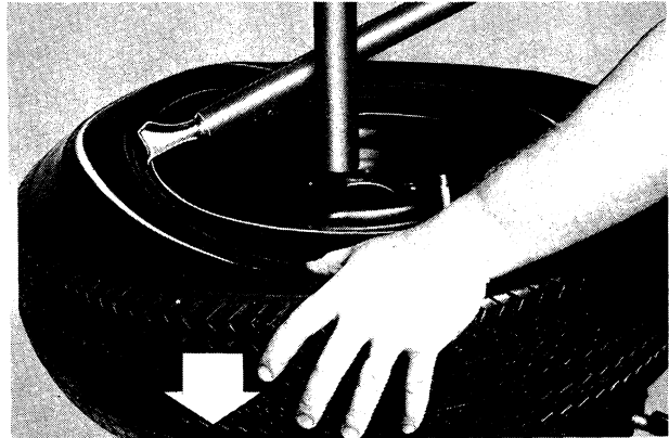
5. Apply rubber lubricant to both beads. Position the mounting end of the combination tool through the pivot arm as shown and hook the end over the rim. Place the lower bead over the hook and against the shoulder of the tool. Start bead in drop center with hand and rotate the tool clockwise until the first bead is mounted. Note: The tool is optimized to work best held at approximately 30° to the wheel as shown.
