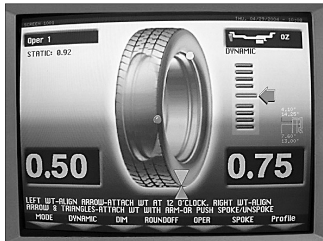
Figure 17 - Weight Placement Arrows in 3D Mode.
