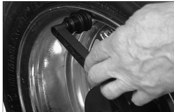
Figure 52 - Diameter Arm (Plastic) Calibration
