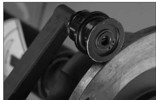
Figure 49A - Plastic Offset Arm Gauge to Faceplate
