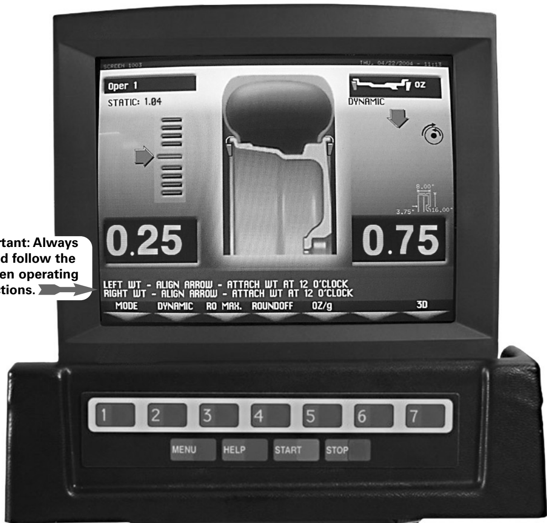
Figure 3 - Weight Placement Screen Using Clip-on Weights in Dynamic Mode
