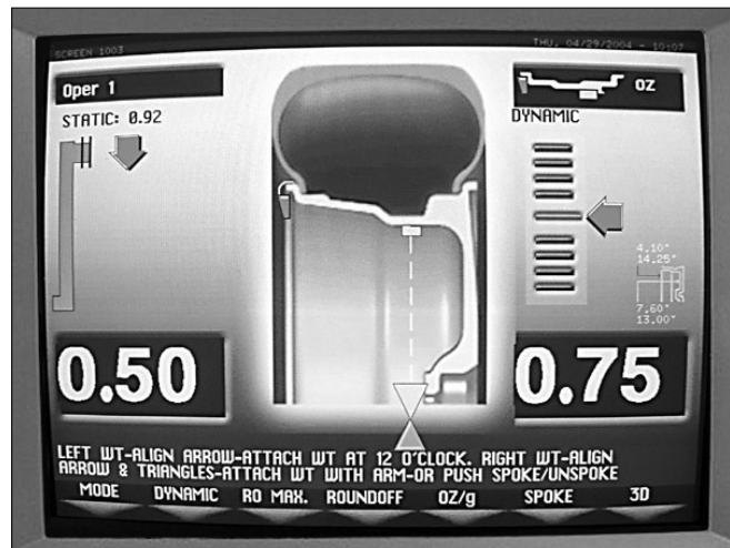
Figure 18 - Weight Placement Arrows in Profile Mode.
