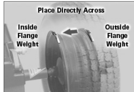
Figure 46A - Test Weight Inside Flange Position
