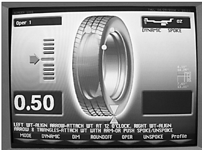
Figure 28 - Spoke Weight Placement Screen
