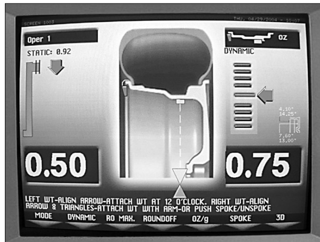
Figure 15 - Weight Placement Arrows in Profile Mode.
