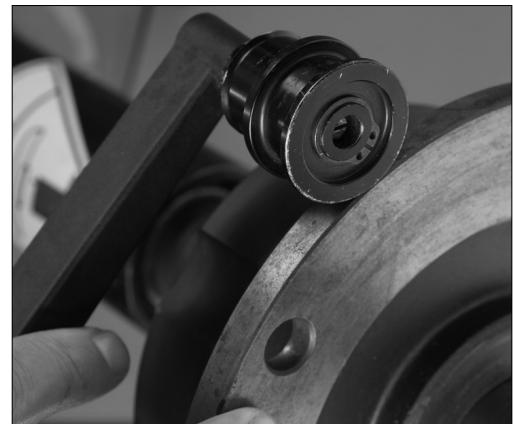
Figure 40 - Offset Arm Gauge to Faceplate
