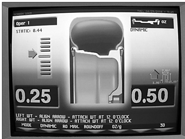
Figure 25 - Clip-on Weight Placement Screen
