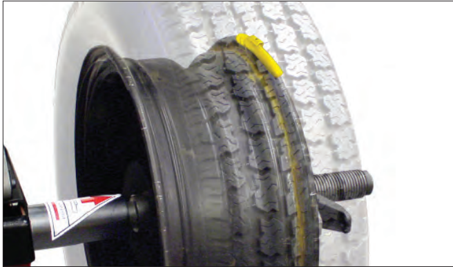
Figure 1 - Calibration Weight On Outside Flange At Top-Dead-Center
