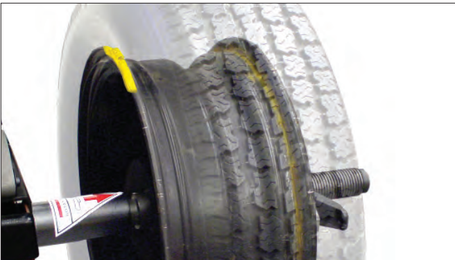
Figure 2 - Calibration Weight Moved (Directly Across) To Inside Flange
