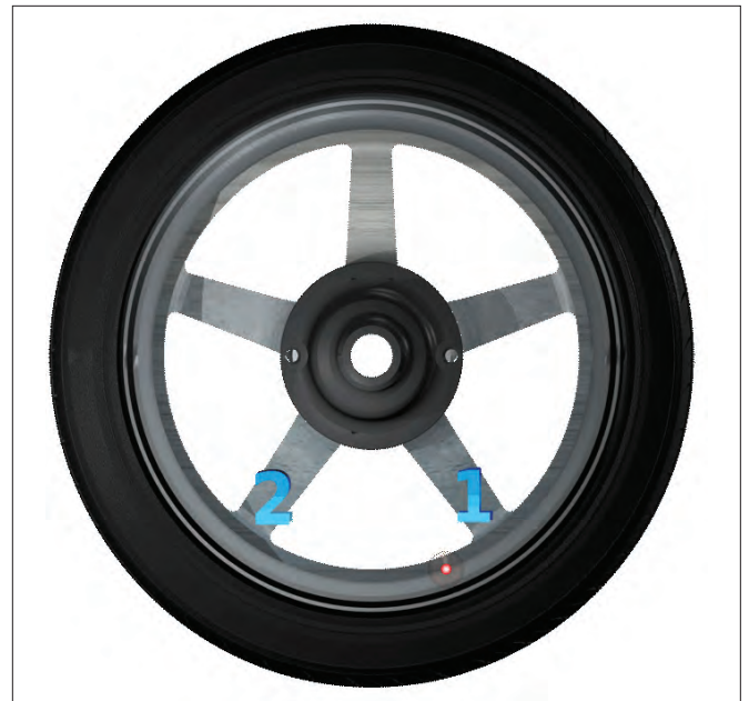
Figure 25 - Spoke 1 and Spoke 2 Locations On Either Side Of Original Outboard Weight Location
