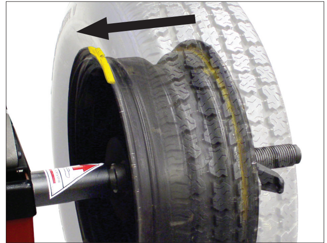
Figure 21 - Calibration Weight Moved (Directly Across) To Inside Flange
