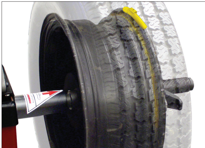
Figure 20 - Calibration Weight On Outside Flange At Top-Dead-Center
