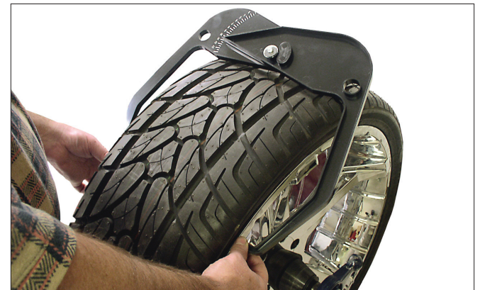
Figure 13 - Caliper Placement On Wheel
