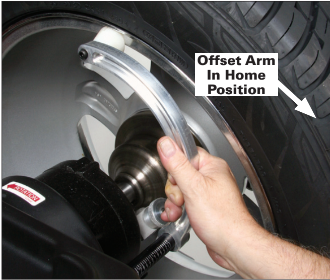
Figure 6A - Automatic A&D Measurement At Clip-on Weight Location
