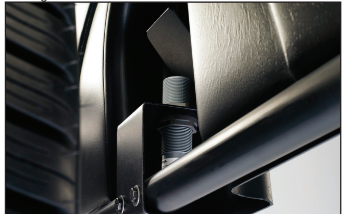
Figure 10 - Tire Width Sonar Located Inside Hood
