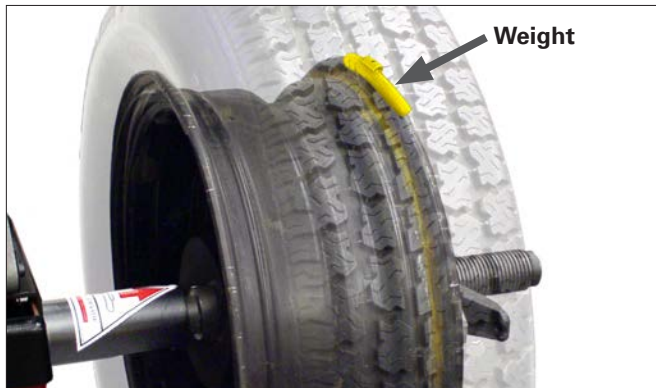
Figure 40 - Calibration Weight On Outside Flange At Top-Dead-Center
