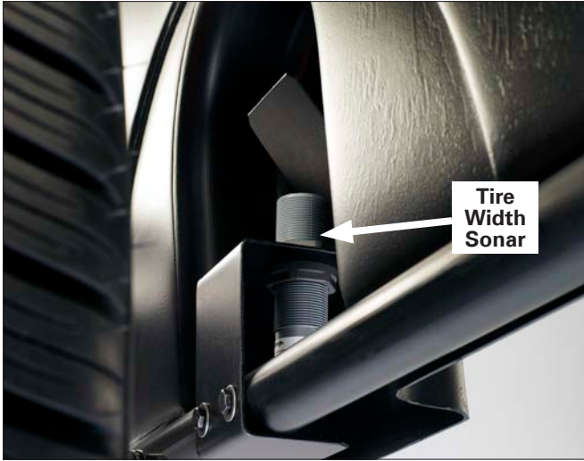
Figure 18 - Tire Width Sonar Located Inside Hood
