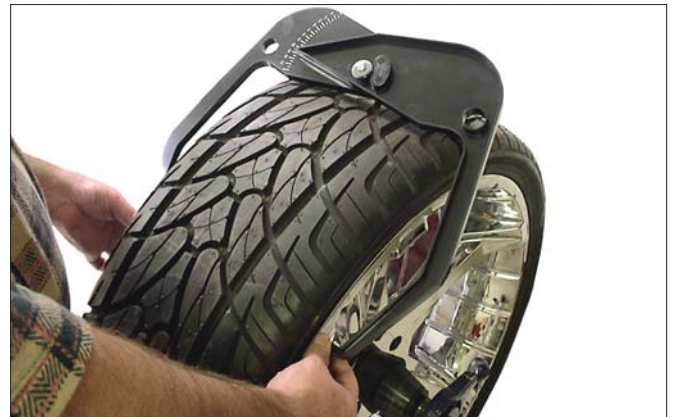
Figure 19 - Caliper Placement On Wheel
