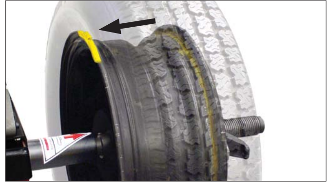
Figure 25 - Calibration Weight On Inboard Flange At Top-Dead-Center
