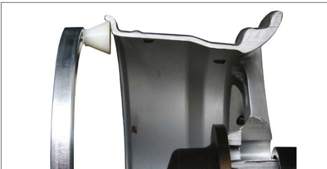
Figure 2 - Clip-On Weight Location
