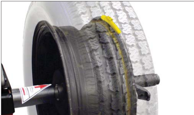
Figure 24 - Calibration Weight On Outboard Flange At Top-Dead-Center
