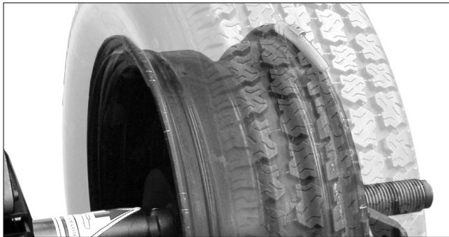
Figure 19 - Calibration Weight On Outside Flange At Top-Dead-Center
