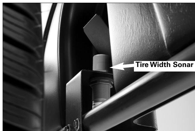
Figure 10 - Tire Width Sonar Located Inside Hood
