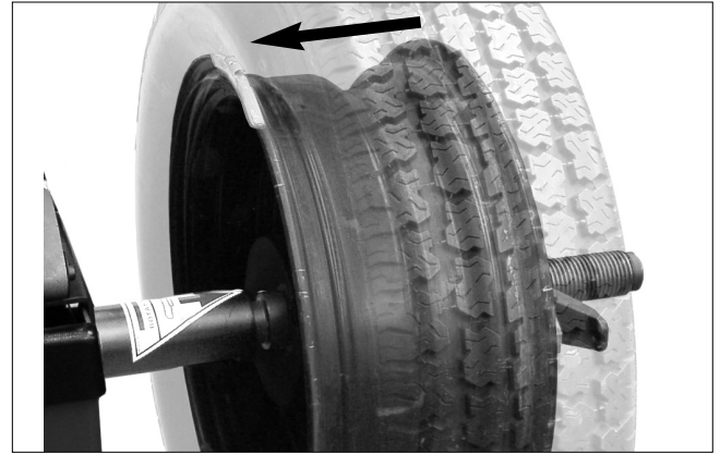
Figure 21 - Calibration Weight Moved (Directly Across) To Inside Flange
