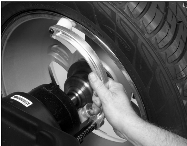
Figure 6A - Automatic A&D Measurement At Clip-on Weight Location
