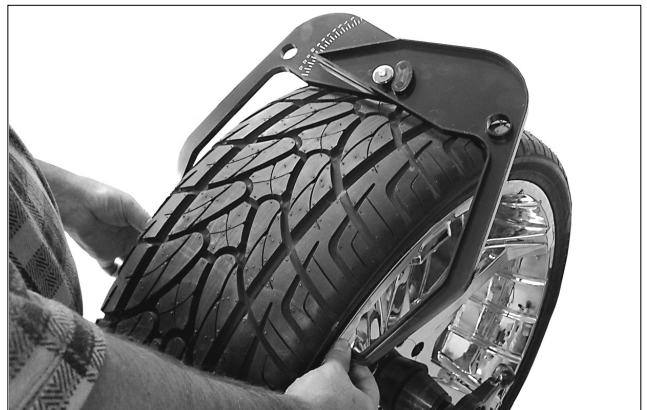
Figure 13 - Caliper Placement On Wheel
