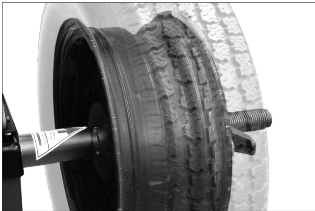
Figure 20 - Calibration Weight On Outside Flange At Top-Dead-Center
