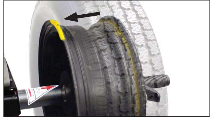
Figure 25 - Calibration Weight On Inboard Flange At Top-Dead-Center
