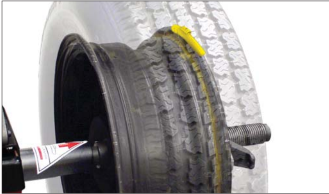
Figure 24 - Calibration Weight On Outboard Flange At Top-Dead-Center
