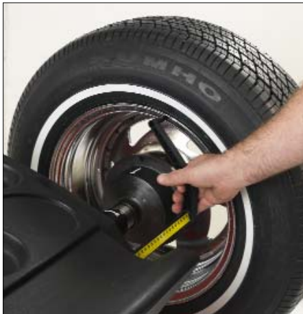
Figure 3 - Offset Arm At Clip-On Weight Location
