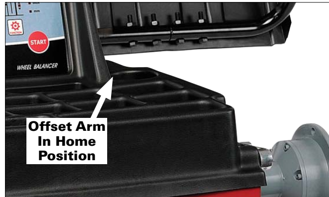
Figure 7 - Offset Arm Stored In Home Position
