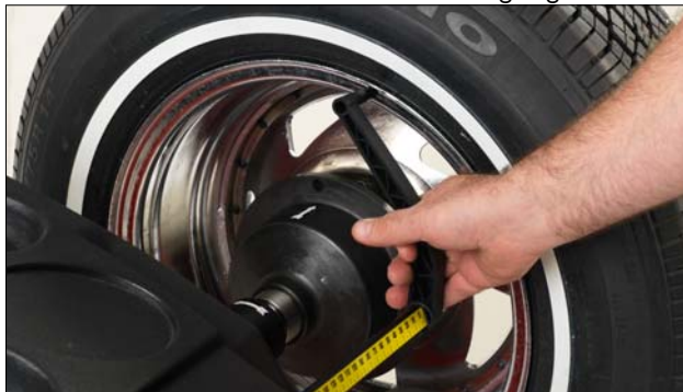
Figure 13 - Offset Arm at Clip-on Weight Location
