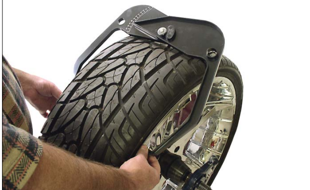
Figure 12 - Caliper Placement On Wheel
