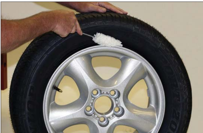
Figure 5 - Apply Rubber Lubricant to Tire Beads
