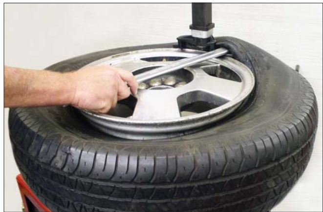
Figure 11 - Holding Lifting Tool in Place and Rotate Wheel
