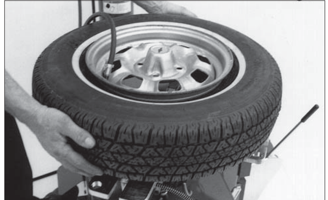
Figure 19 - Lift Tire Upwards for Bead Sealing
