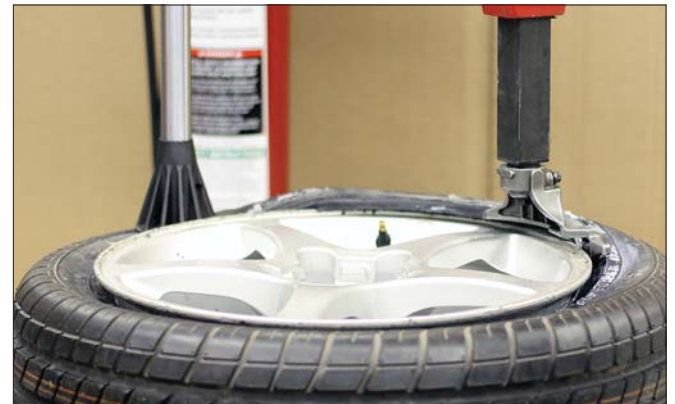
Figure 15 - Assist Foot to Flip Bead Over Rim Flange
