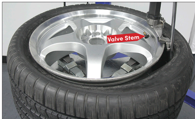
Figure 13 - Insert Bead Lifting Tool Below Tire Bead
