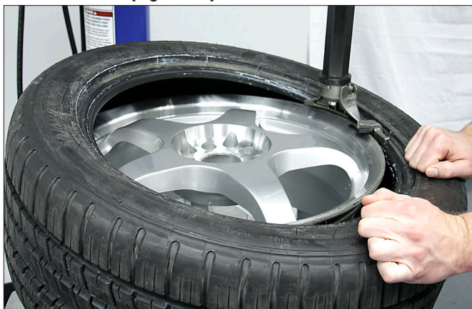
Figure 21 - Mounting Top Bead
