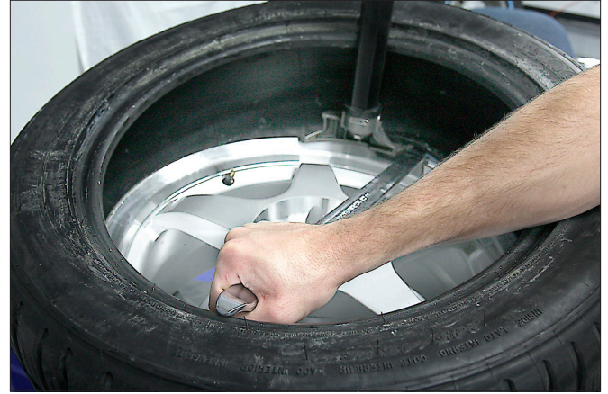
Figure 16 - Guide Lower Bead Over Tool Knob
