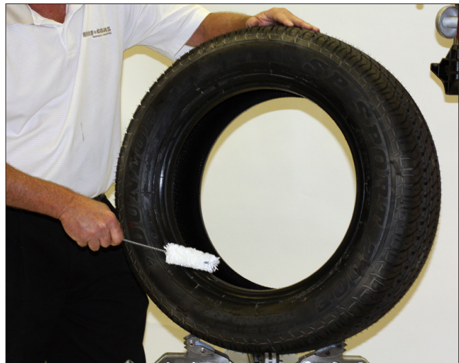
Figure 19 - Lubricate Tire Beads Liberally
