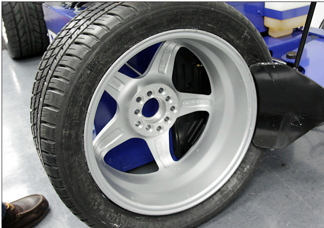
Figure 7 - Position Tire and Bead Loosener Shoe With Wheel Turned Around
