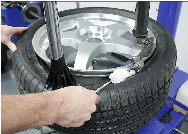
Figure 26 - Lubricate Upper Bead
