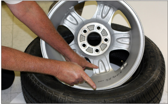
Figure 17 - Verify Size Match Between Tire and Wheel
