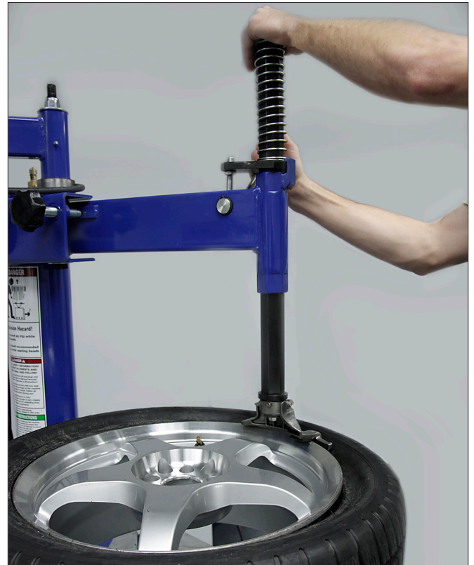
Figure 10 - Position Mount/Demount Tool.
