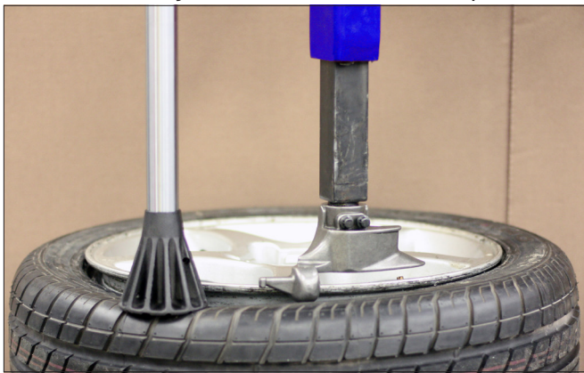
Figure 25 - Helper Arm Foot Depressing Sidewall of Tire
