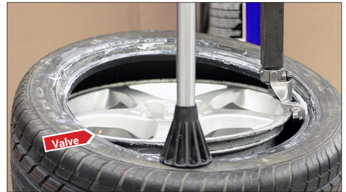
Figure 32 - Mount Upper Tire Bead, Use Helper Arm
