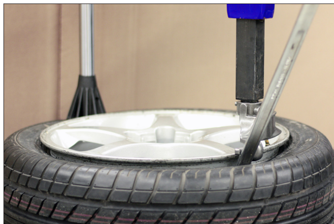
Figure 28 - Insert Bead Lifting Tool
