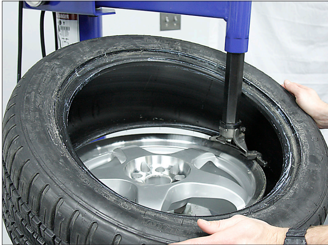
Figure 20 - Position Tire Against Mount/Demount Tool
