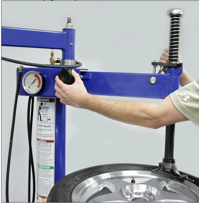
Figure 11 - Adjust Swing Arm to Position Tool Roller
