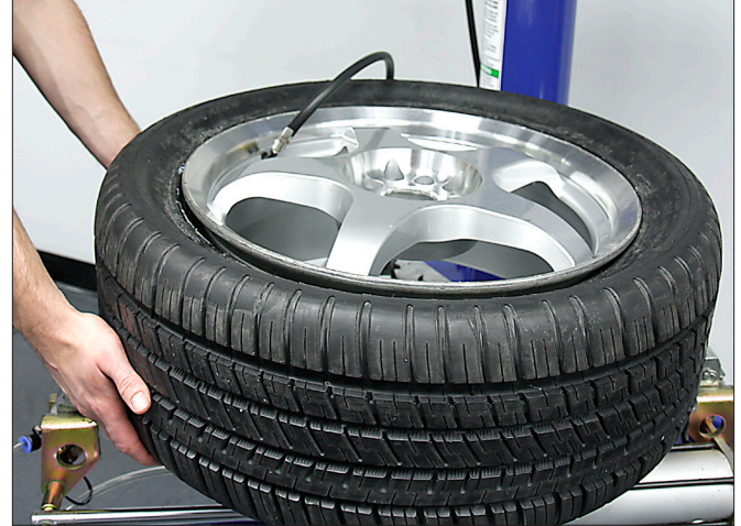
Figure 22 - Lift Tire Upwards for Bead Sealing
