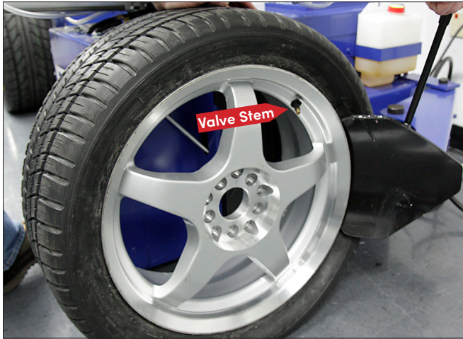
Figure 6 - Position Tire and Bead Loosener Shoe
