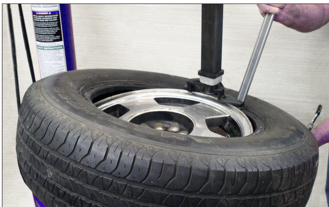
Figure 31 - Lower Tire Bead in Drop Center
