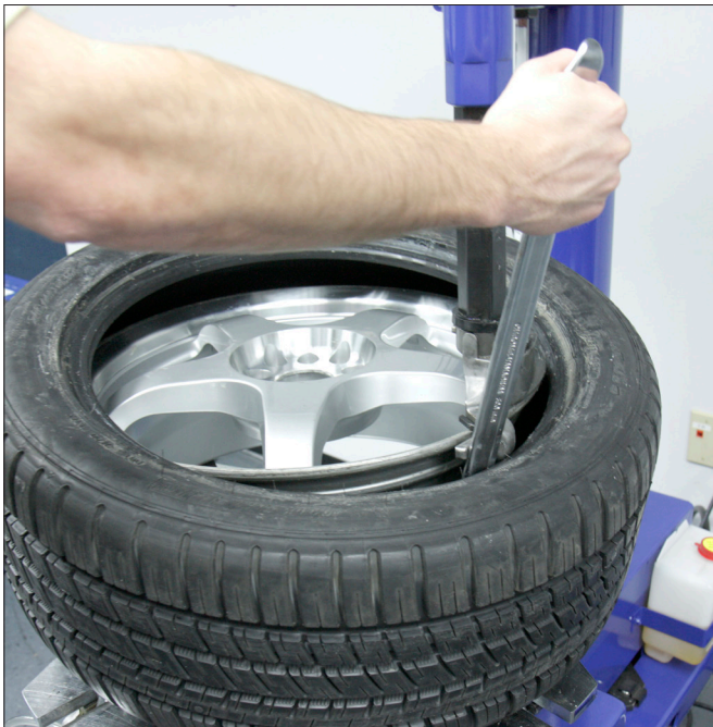
Figure 15 - Demounting Lower Bead
