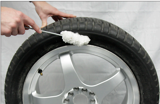
Figure 8 - Apply Rubber Lubricant to Tire Beads
