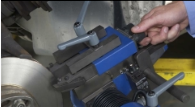
Adjust the opposite carbide insert in the same manner.
