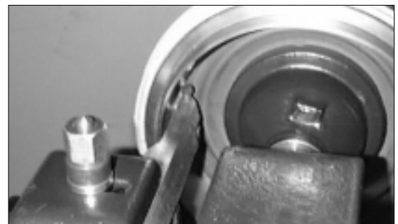
Figure 9 - Positioning the Boring Bar
