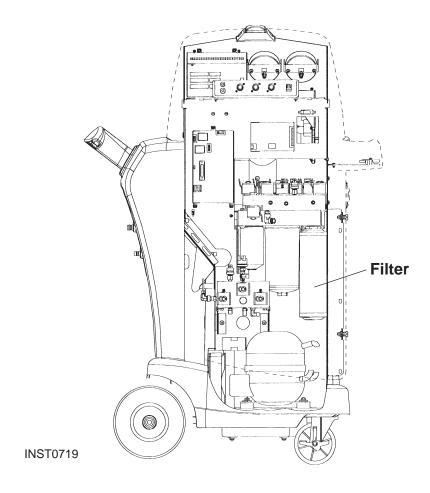
**CAUTION!** The filter change process should not be done with the unit connected to the vehicle. Disconnect the unit by closing the service coupler valves and disconnecting the high and low side hoses from the vehicle.
